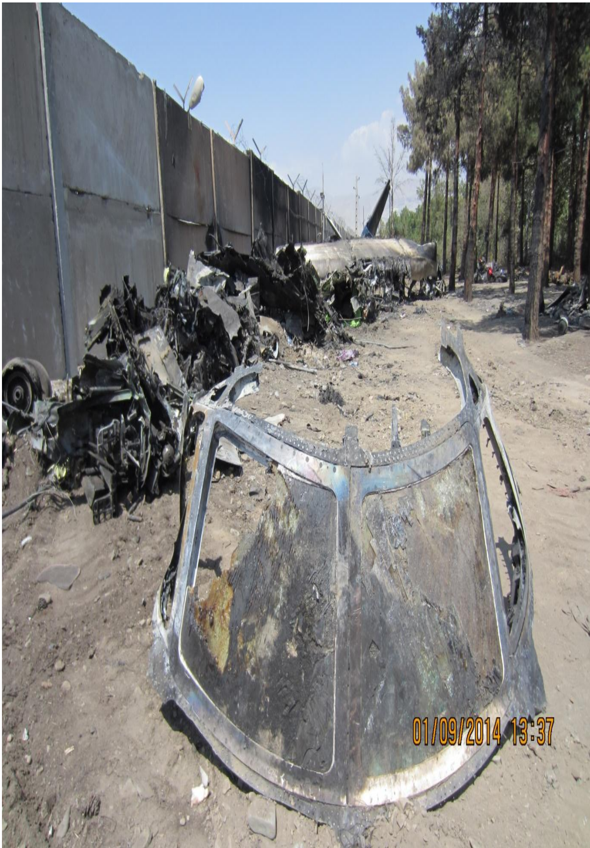
Figure 17. Fire damage to the fuselage
