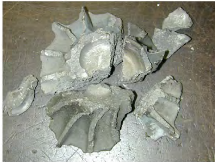
Photo 1: Turbine wheel broken into several pieces (American)
