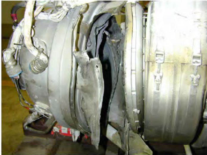
Photo 2: External view of APU showing ruptured compressor case (American)
