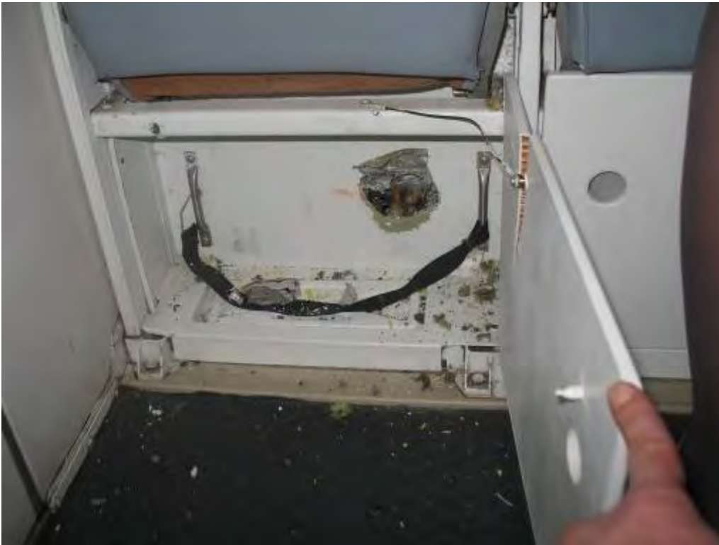
Image 5: Punctured bulkhead below the right aft flight attendant seat Fracture piece of the compressor wheel in the bottom of the bin
