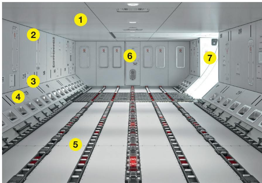
“ The air-tight lining of the cargo compartment is created by composite panels together with their fasteners, secondary structure and the cargo door. ”
