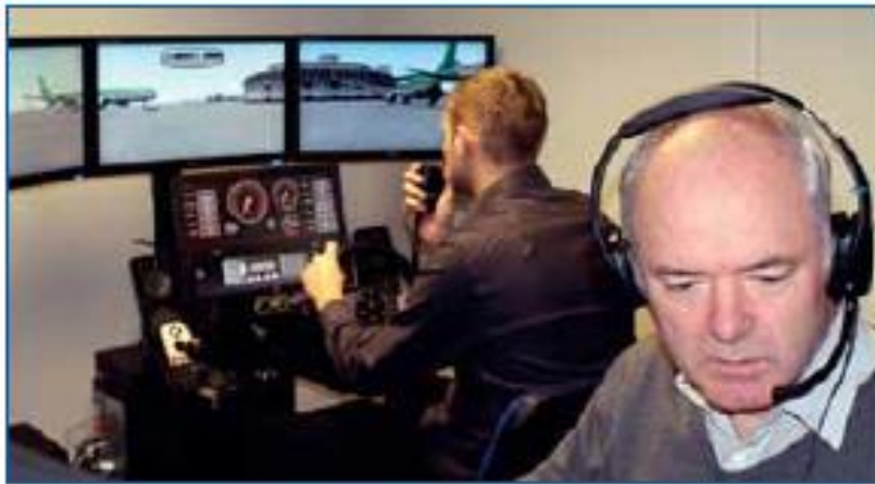
An instructor working with a trainee driver. The instructor has an intuitive touch-screen interface to control background radio conversations.
