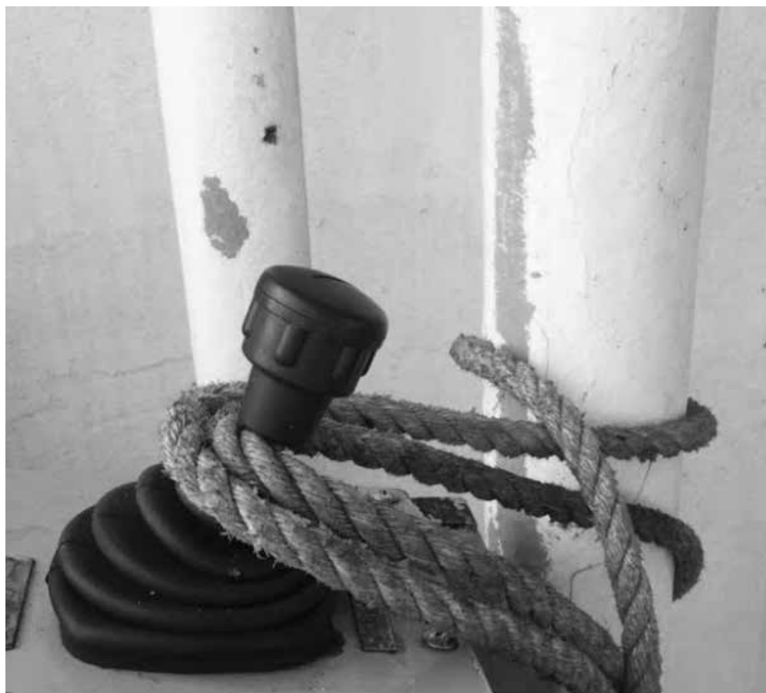
Figure 1: Winch control lever tied with a rope
