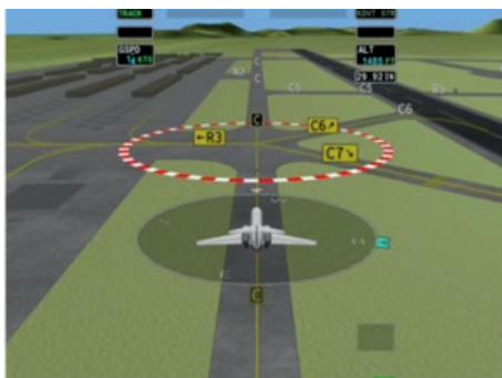
Figure 26: 3D airport moving map on flight deck primary flight display
