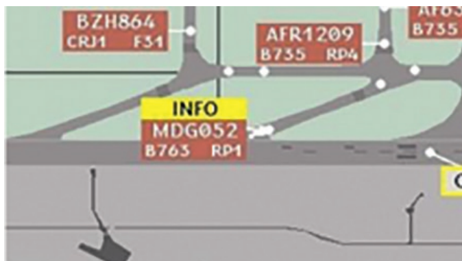
Figure 18: A-SMGCS display when an aircraft is on the runway strip and a car is on the runway
