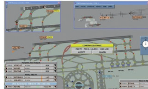
Figure 21: Pop-up window in centre asks for confirmation of apparent conflicting clearances
