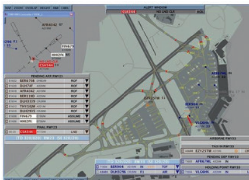
Figure 22: Red highlight appears in alert window at top of display and red highlight on ATM element and arrivals elements for aircraft with no landing clearance within 1 mile
