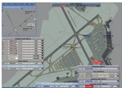
Figure 23: Red highlight appears in alert window at top of display and red highlight in holding point bay and runway entry point for an aircraft which is entering the runway without a clearance
