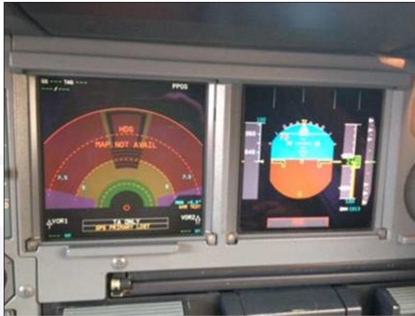
Figure 10-Weather radar antenna scanning operational test.
