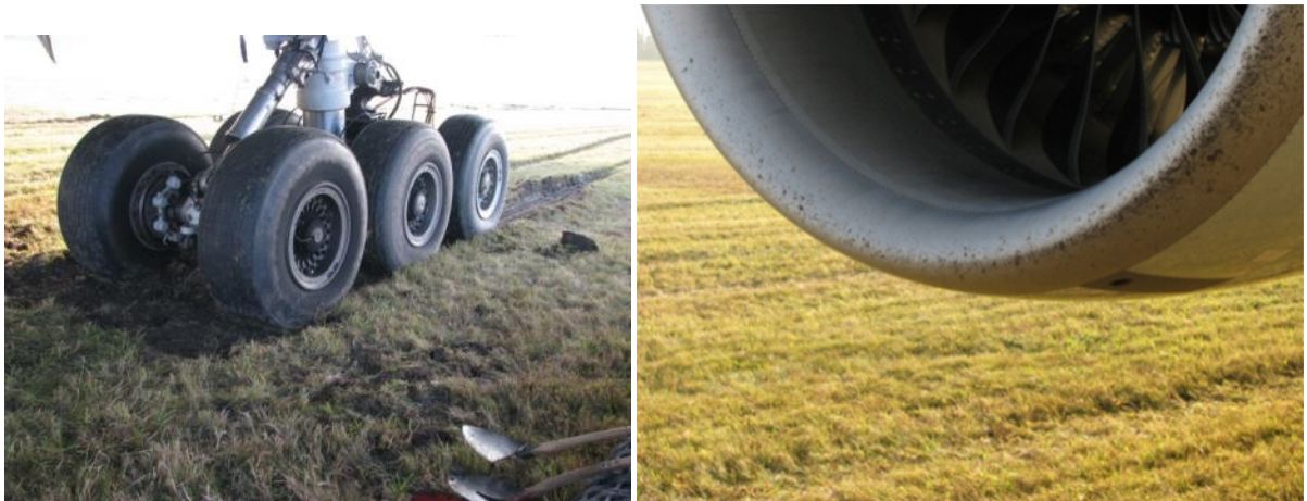
Right main landing gear and contamination on the right engine
