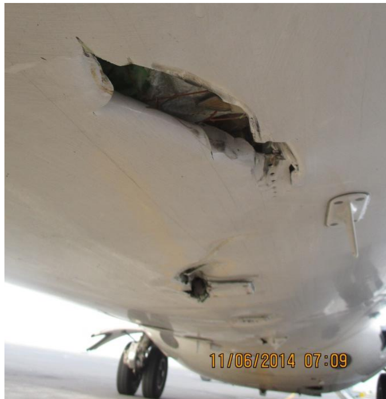
Figure 3: Damages found on the lower fuselage
