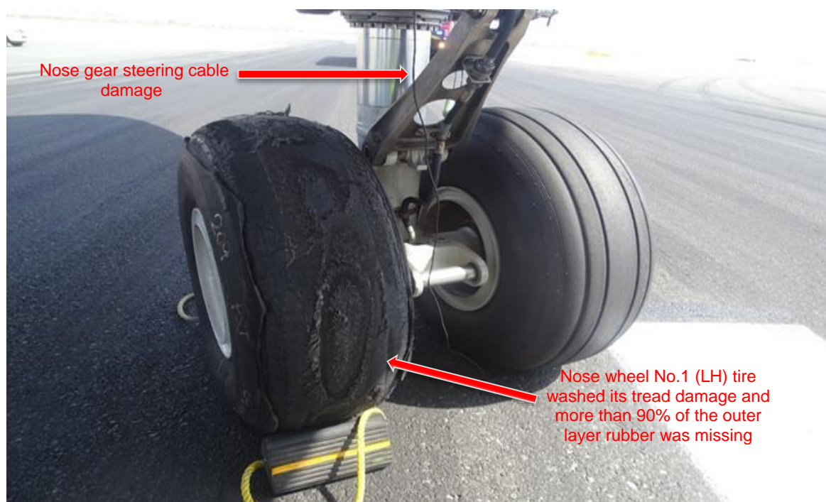
Figure 4. No.1 nose wheel tire and steering cable damage
