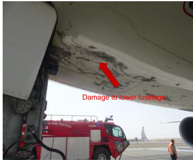
Figure 5. Damage to lower fuselage aft of the NLG bay
