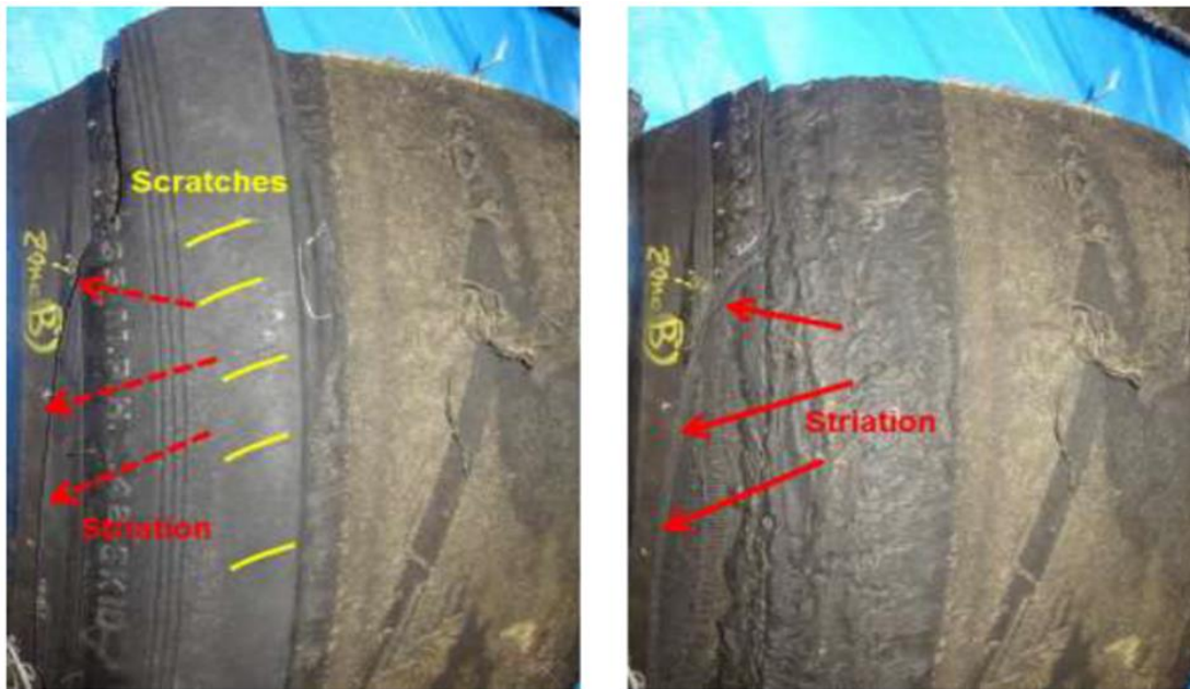
Figure 16. Damaged tire, zone B
