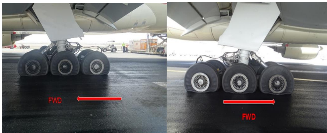
Figure 3. MLG wheels (LH & RH) deflated
