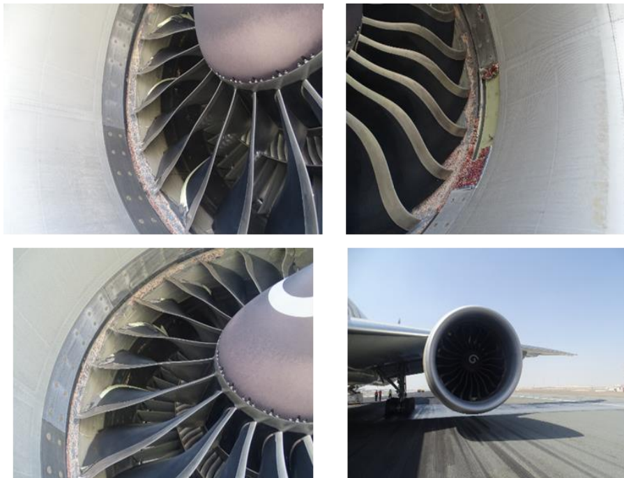
Figure 6. LH engine fan blades and Inlet damage
