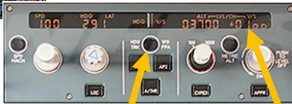
Vertical Speed/Flight Path Angle Selector Switch
