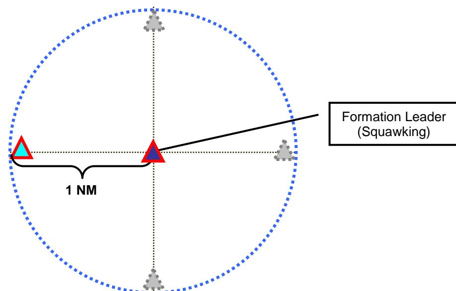
A Standard Military Formation, usually consisting of 2 to 4 aircraft will remain within a cylinder-shaped airspace of 1 NM radius and 200 ft height, defined by the squawking aircraft (formation leader), representing the center of the cylinder.
