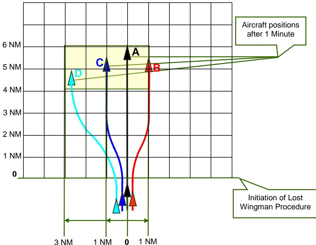
After completion of the lost wingman procedure, all aircraft will continue to comply with the previous clearance issued for the formation until instructed otherwise, however, as shown above, spread out in an area of approximately 2 by 4 NM and up to 1.000 ft in height.
