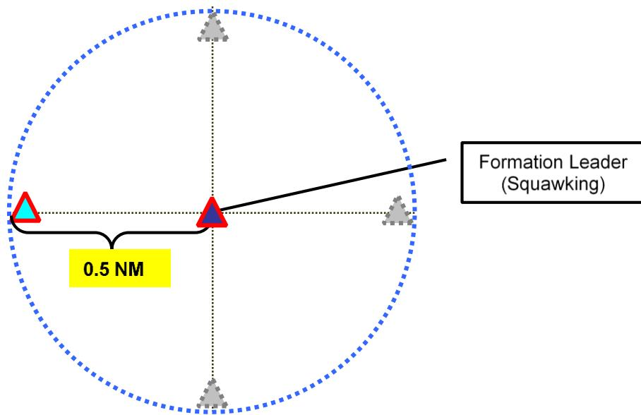
A Standard Military Formation, usually consisting of 2 to 4 aircraft, shall remain within a cylinder-shaped airspace of max 0.5 NM radius and max 200 ft height, defined by the squawking aircraft (formation leader), representing the center of the cylinder.
