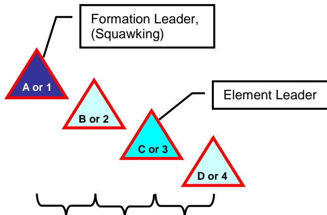
Usually from 3 feet wingtip-clearance to 2-4 aircraft-widths spacing between individual aircraft
