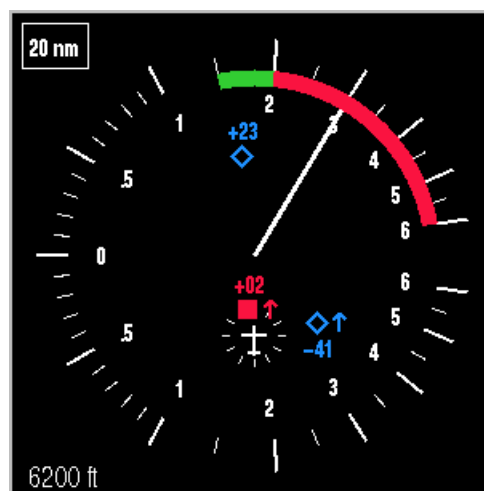
Figure 23: 14 th April 2006 event - IVSI for lower TCAS aircraft
