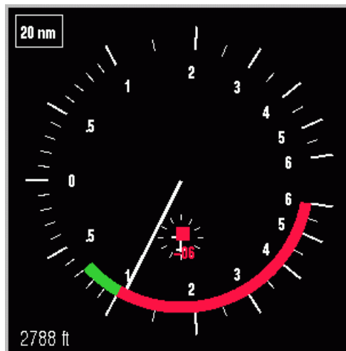
Figure 16: 30 th March 2006 event - IVSI onboard TCAS aircraft
