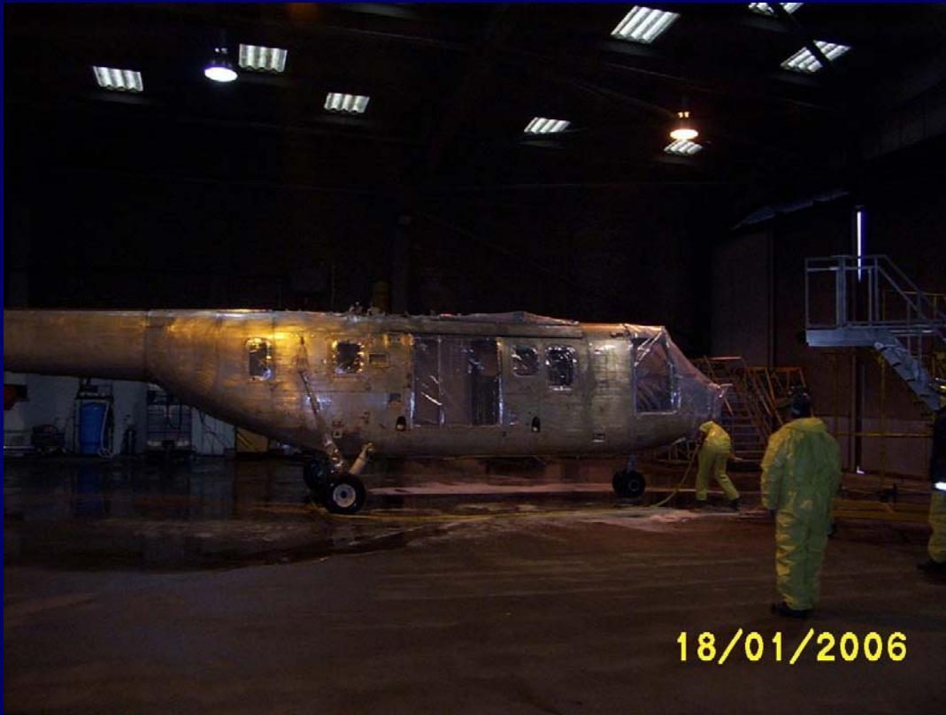
G-TIGE paint stripped, cleaned and awaiting transfer to the maintenance hangar.
