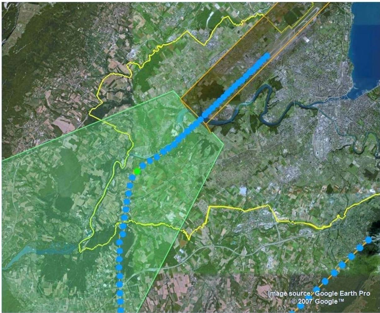
Figure 9-21 DTED alert that is generated when HEADINGTOL is 8°, 10° or 15°, but not when it's 20°
