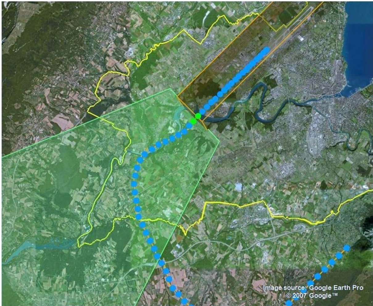
Figure 9-19 DTED alert that is generated when HEADINGTOL is 8° or 10°, but not when it's 15° or 20°
