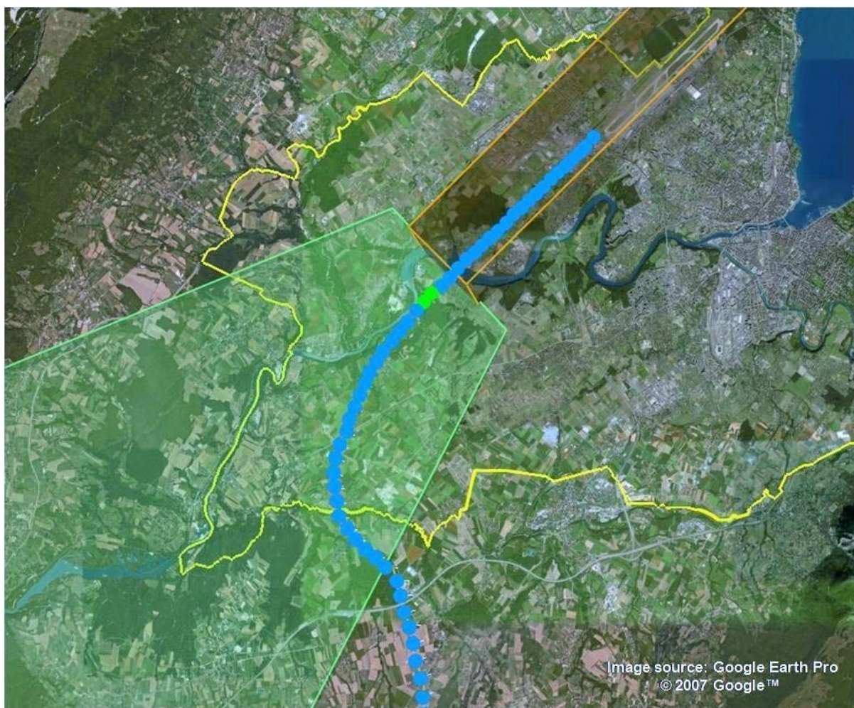
Figure 9-18 Another DTED alert as an aircraft is turning onto the localiser, runway 05
