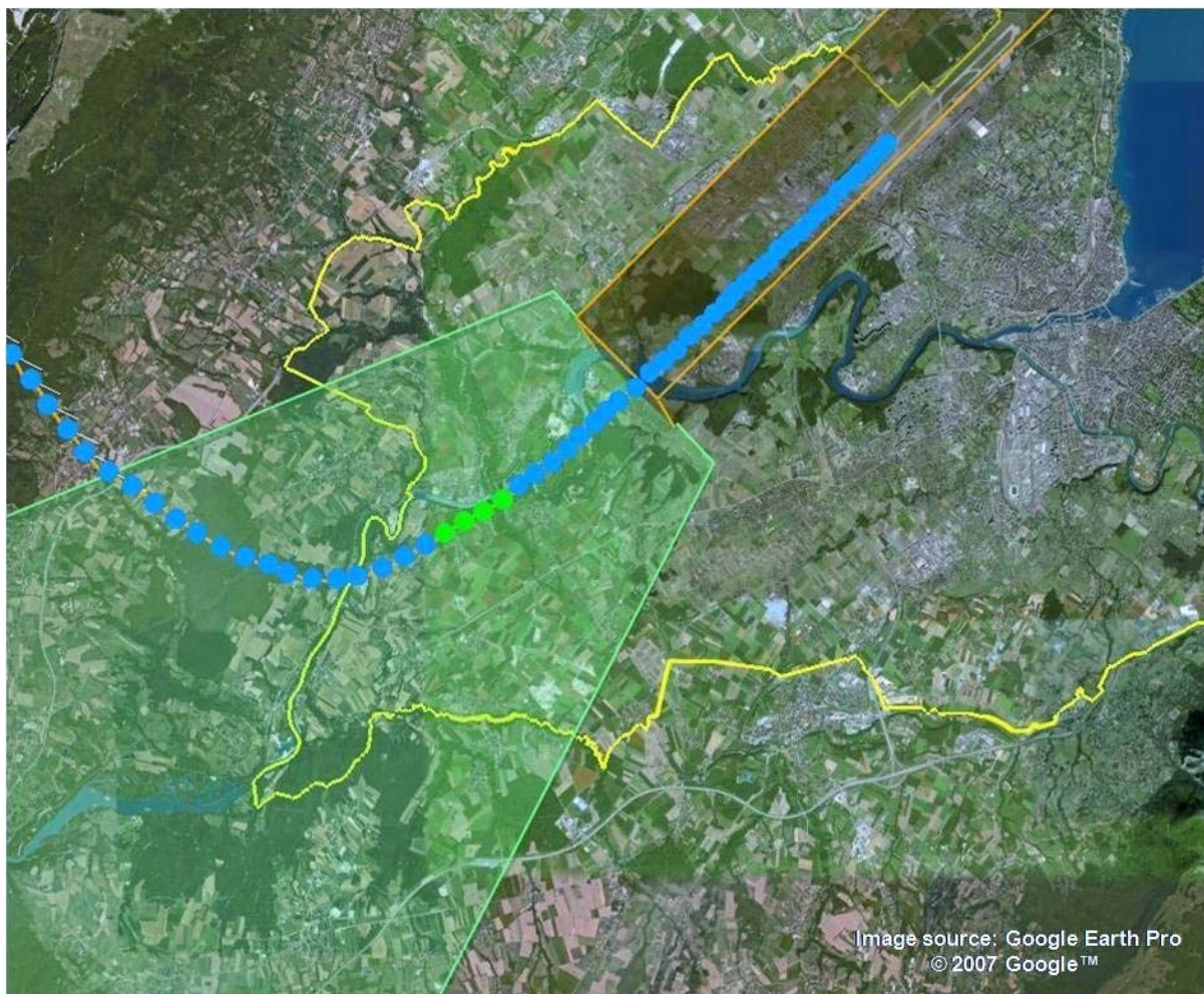
Figure 9-17 A DTED alert as an aircraft is turning onto the localiser, runway 05
