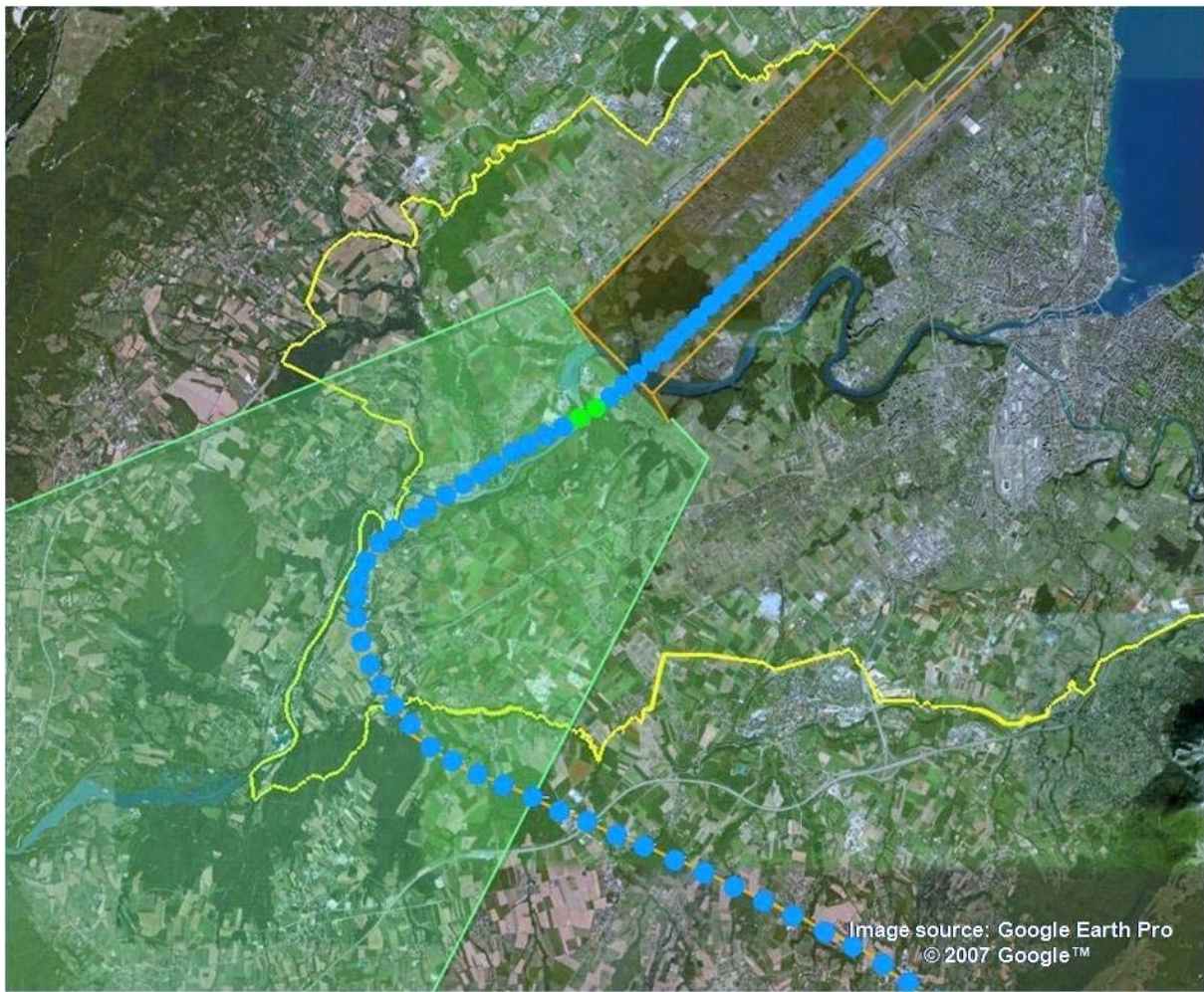
Figure 9-20 DTED alert that is generated when HEADINGTOL is 8° or 10°, but not when it's 15° or 20°
