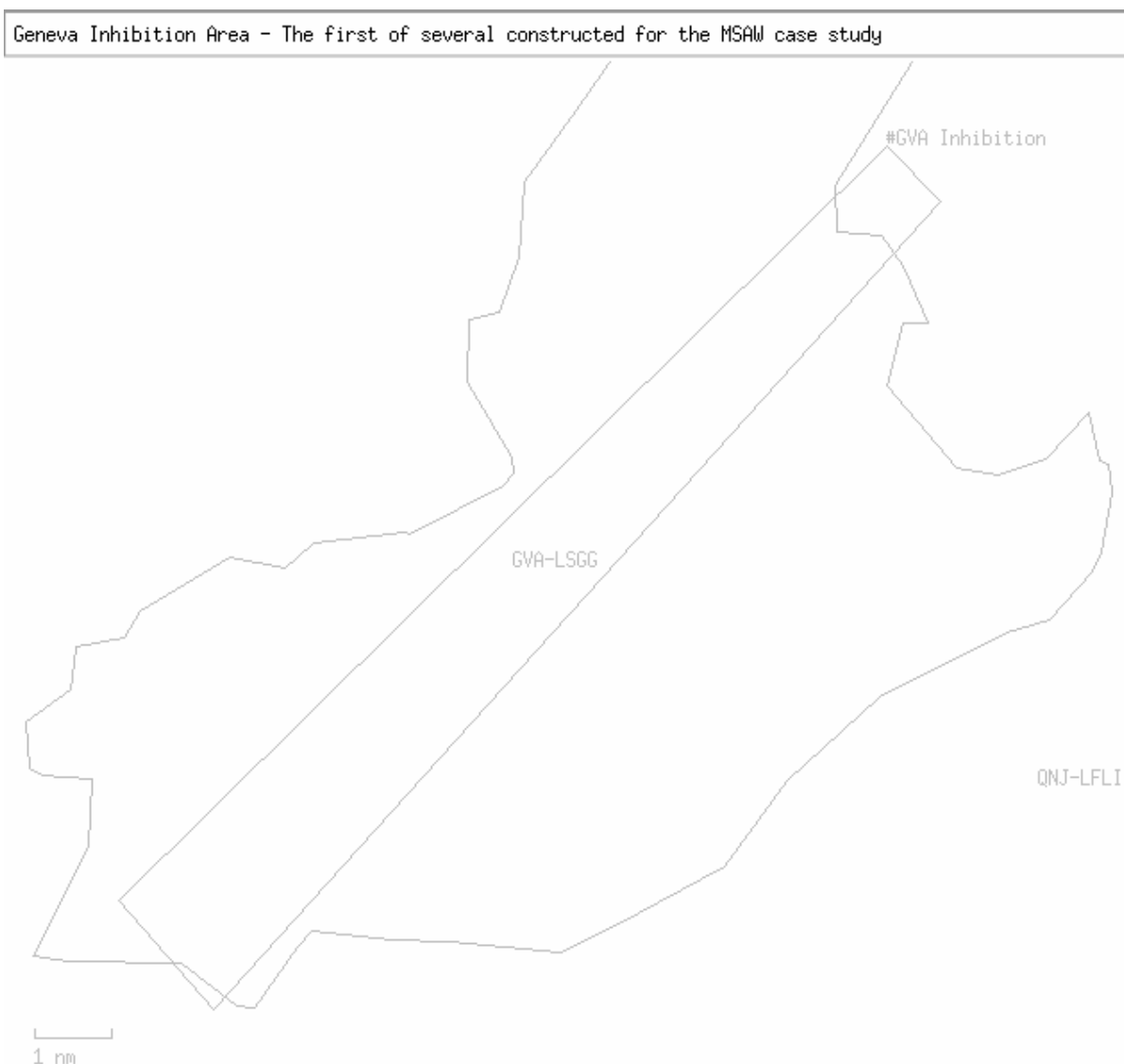
Figure 8-11 MSAW Inhibition Area constructed for Geneva final approach
