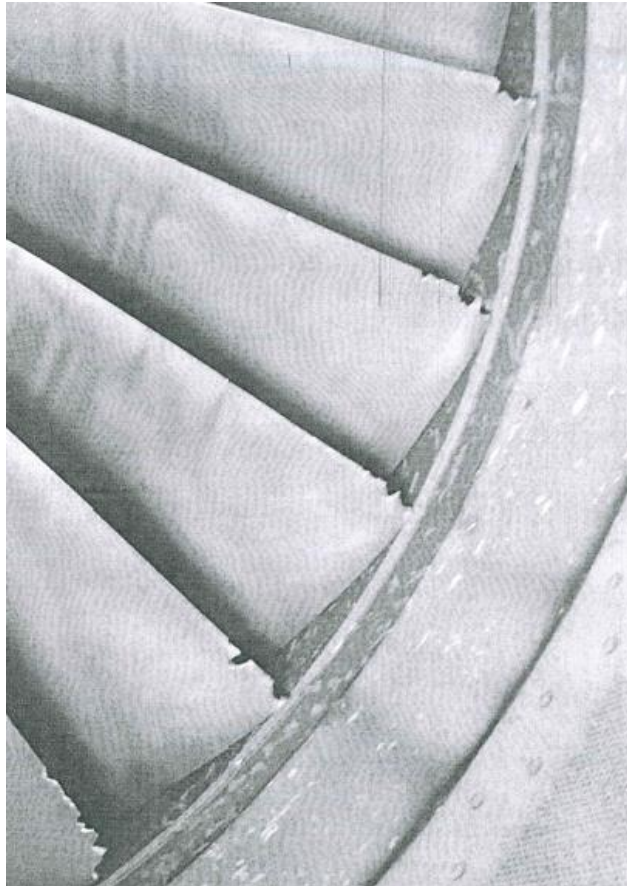
Picture 1: Damage to fan blades of left-hand engine
