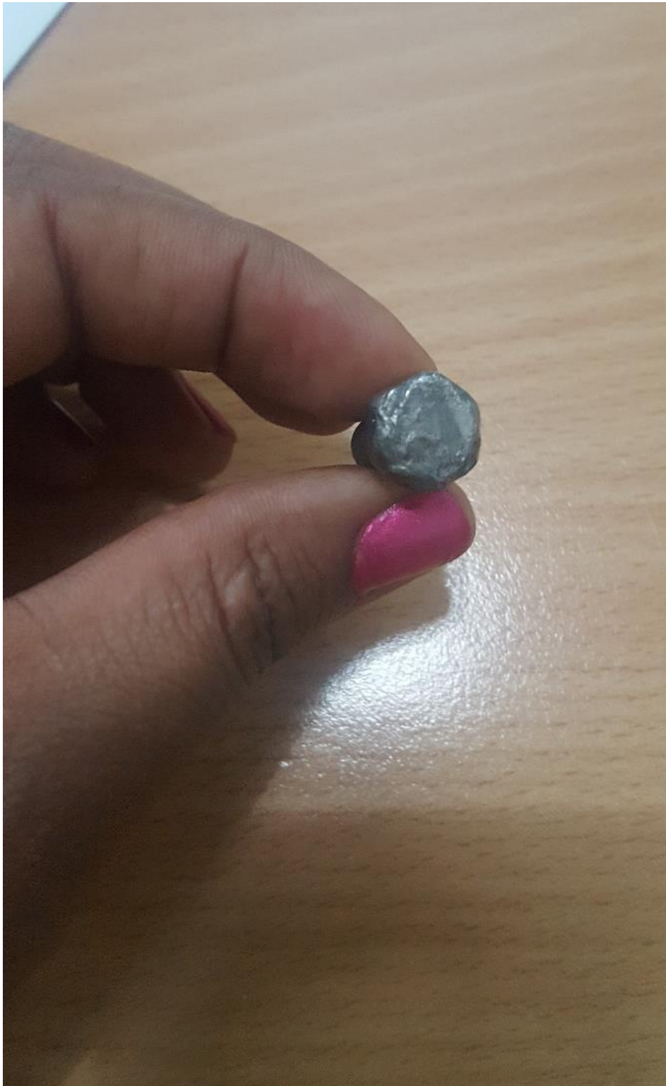
Bolt that was found lodged in acoustic lining of fan intake.
