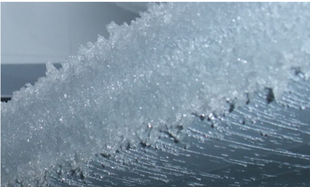
Image 6: Detail of the ice accretion at the wing leading edge
