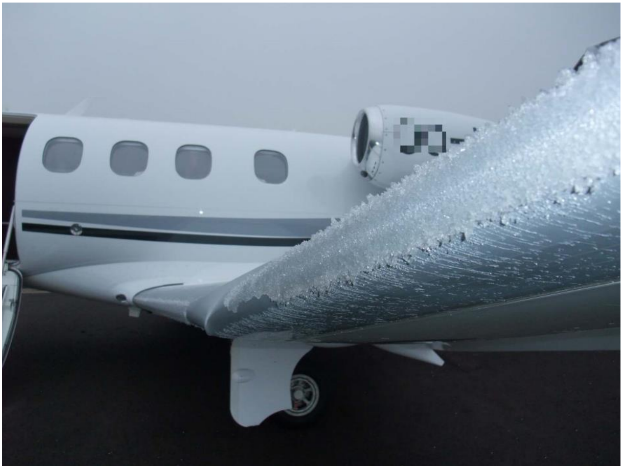
Image 8: Ice accretion about 50 minutes after the accident
