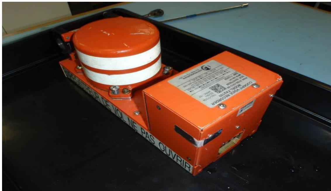
**Figure 4:** Cockpit Voice Recorder
