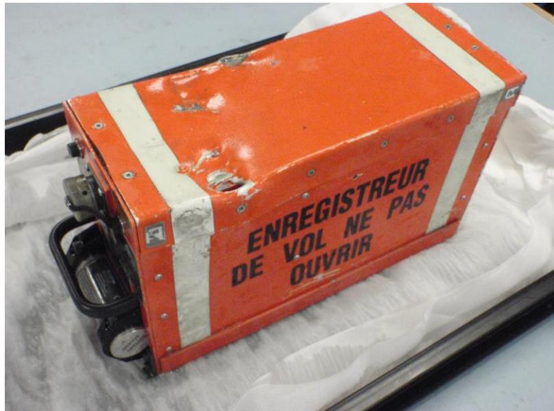
**Figure 2:** Solid-State Combined Voice/Flight Data Recorder
