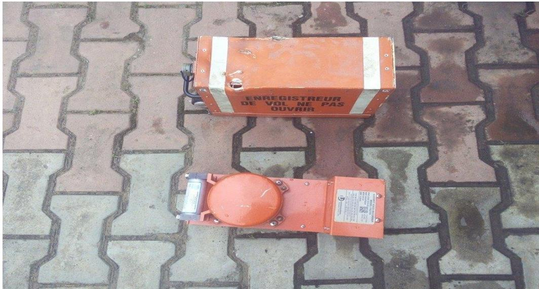
**Figure 3:** The Flight Recorders
