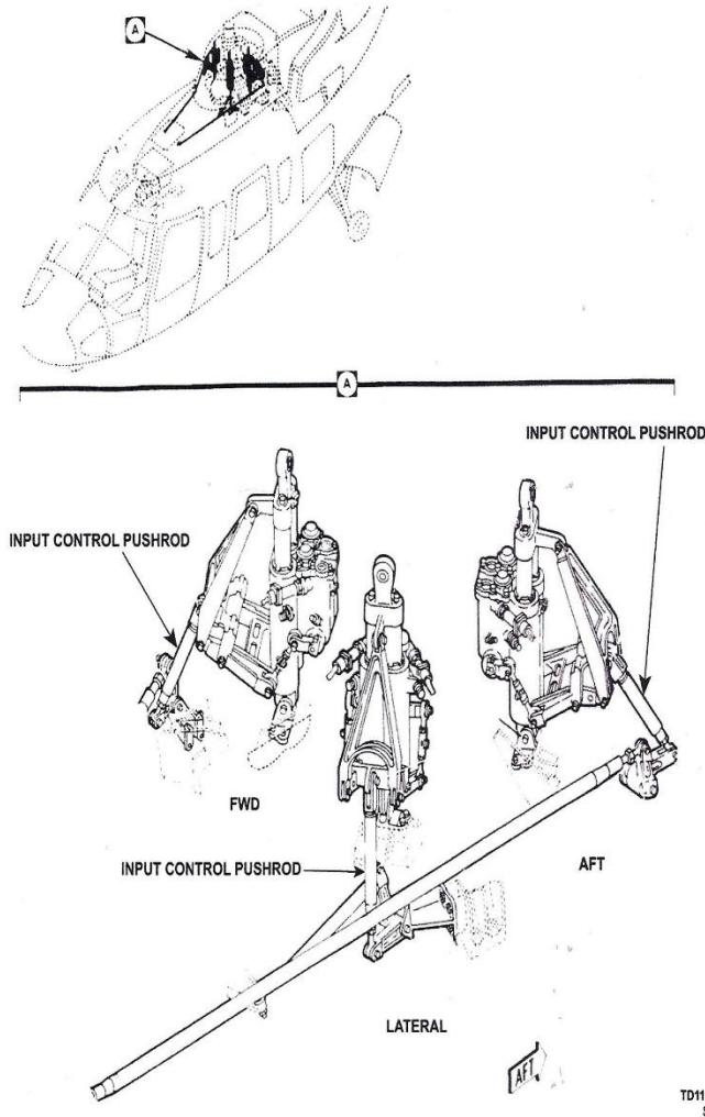
MAIN ROTOR SERVO INPUT CONTROL PUSHRODS
