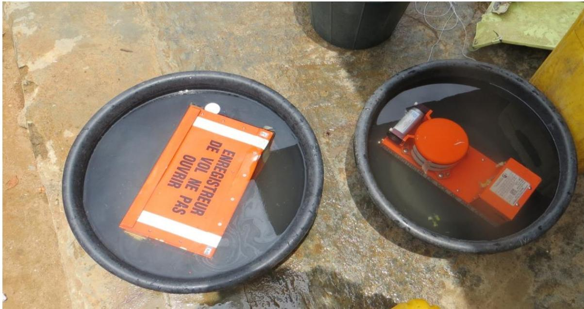
**Figure 5:** Flight Recorders immersed in fresh water for preservation
