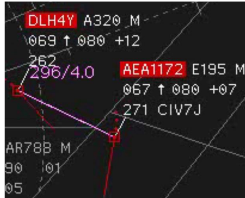
Figure 15: Visualisation of STCA at radar display
