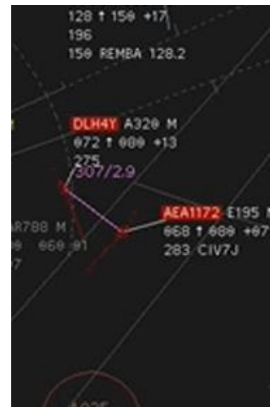
Figure 6: how STCA is shown on radar display
