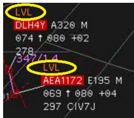
Figure 17: visualisation of the TCAS RA on the radar display
