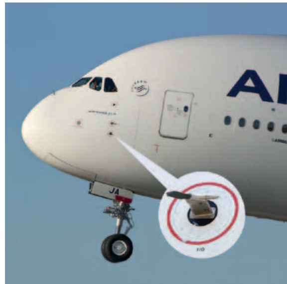
Figure 13 – Pitot-static probes on Air France's Airbus A380
