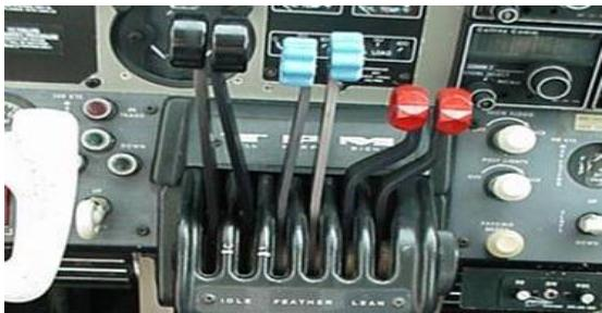
a) **Control.** The first priority is always to fly the aeroplane. Establish control by levelling wings, prevent yaw with rudder and adjust the attitude to achieve and maintain Vyse. (Note that for most light twins Vyse is quoted for maximum all up mass only; at lower mass Vyse is also lower.) Confirm that full power has been selected on all engines and reduce drag by retracting gear and flap.
