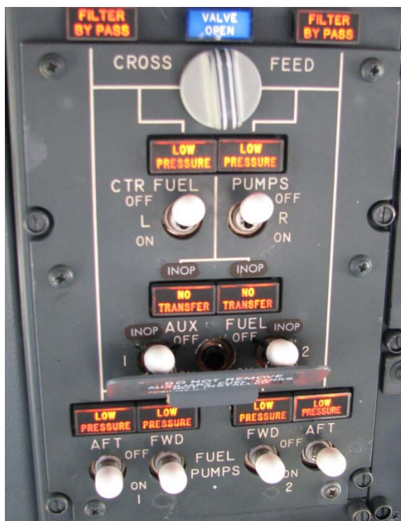
Figure 2: Overhead fuel control panel of VH-TJE photographed from the pilot in command's seat
