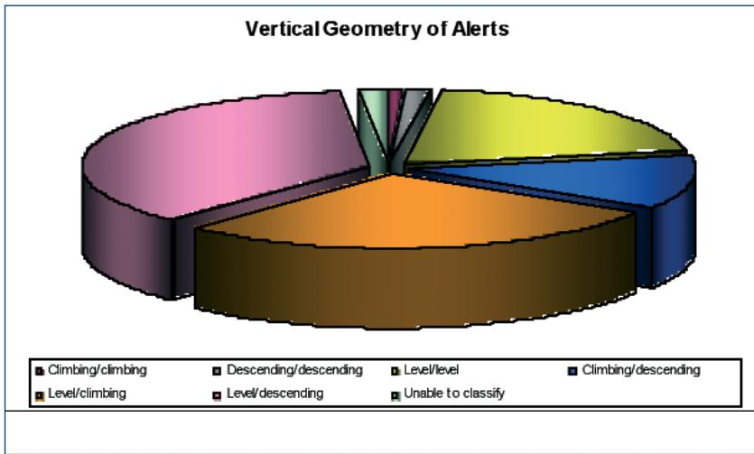
Combining the lateral and vertical geometries of the alerts shows that approximately 80% of crossing encounters involved one or both aircraft that were climbing or descending.
