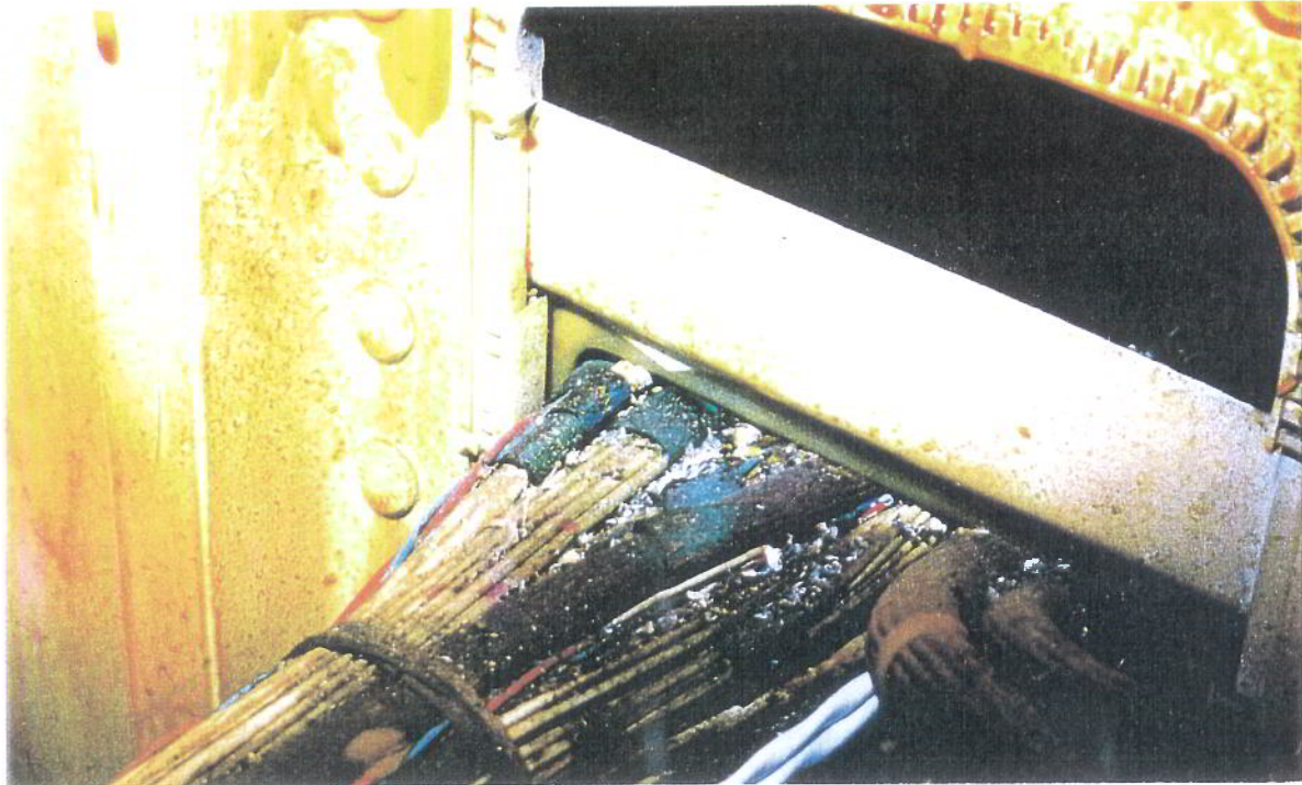
Contamination of wiring looms by drilling swarf, found in a retired B747, above, and an A300, below.
