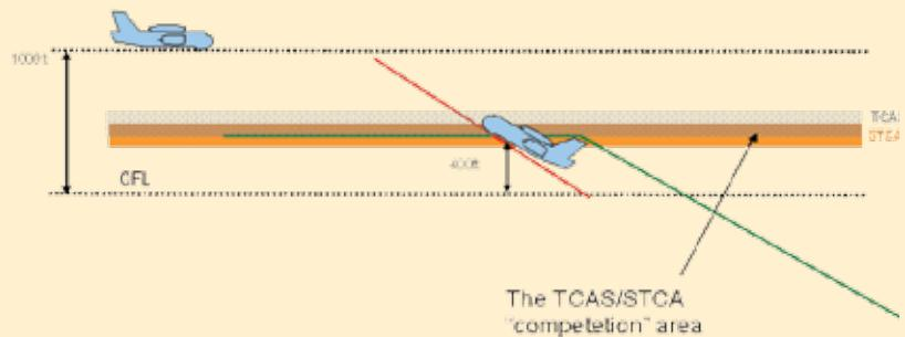
As discussion of our example has shown, there is a discrepancy between what the controller sees and the actual position of the aircraft because of the finite radar refresh rate. This is often forgotten in a moment of high stress.
