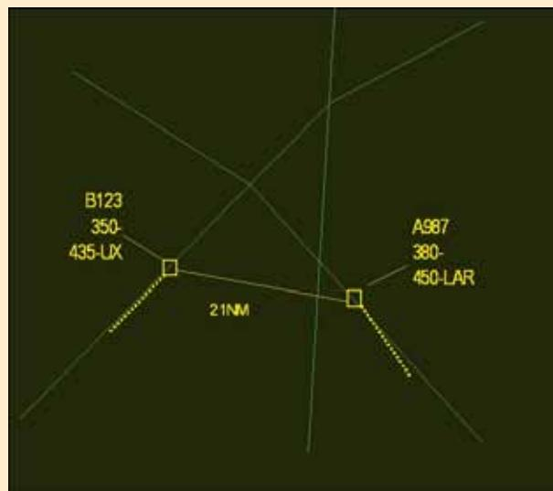
3. A987 actually descends to FL340 (due to an altitude restriction erroneously entered in its FMS) and does not tell the ATCO
