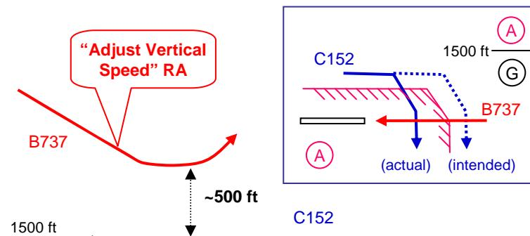
**To improve flight safety, VFR traffic should operate an altitude reporting transponder in all airspace classes, including Class G.**
