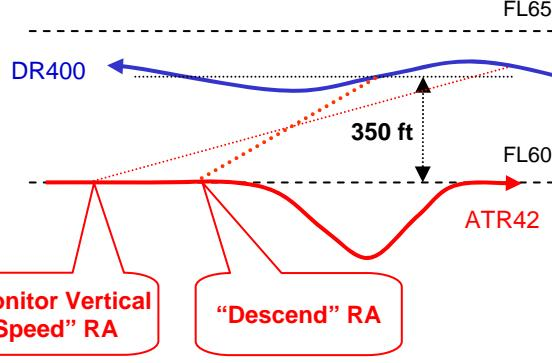
Subsequently, the RA is strengthened into a "**Descend**" RA when the vertical separation between the aircraft becomes less than 350 ft. The pilot follows the RA and descends to FL57 before climbing back to FL60.
