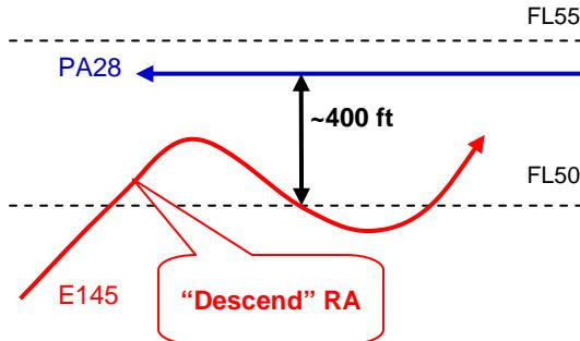
As a result of following the "Descend" RA, the E145 passed about 400 ft below the PA28. Simulations indicate that **without TCAS the separation between the aircraft would have only been about 100 ft and 0.04 NM**.
