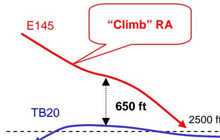
In this event, the high risk of collision resulting from an undetected altimeter setting error was resolved by TCAS, even though the pilot of the E145 did not achieve the vertical speed required by the RA.
