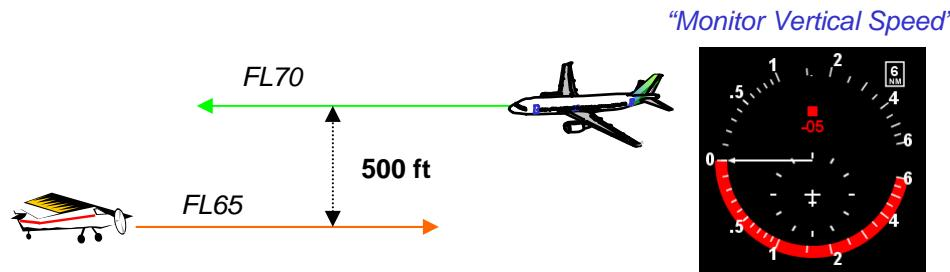
Operational experience shows that **VFR traffic sometimes do not maintain level flight perfectly**. If there is a significant vertical deviation, "Climb" or "Descend" RAs will be generated on-board the TCAS-equipped aircraft.
