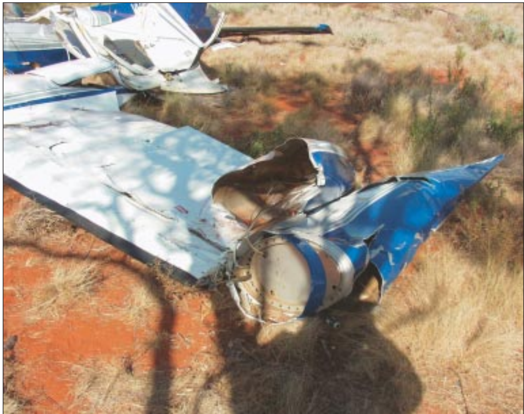
FIGURE 11: Damage to left main fuel tank
