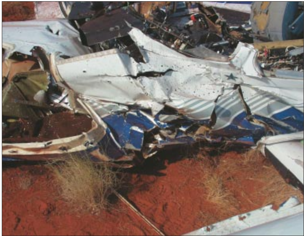
FIGURE 12: Crush damage to forward fuselage section
