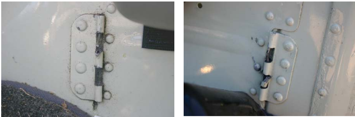
Figure 18: Failed seat belt (airframe) attachments for left front crew seat
