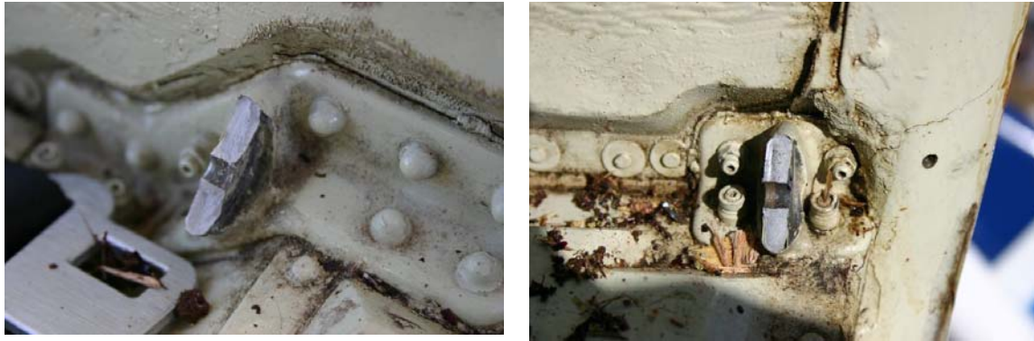
Figure 20: Failed seat belt (airframe) attachments for left rear cabin seat
