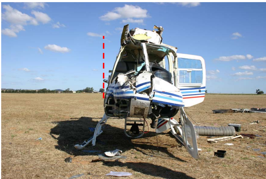
Figure 12: Distortion of fuselage structure
