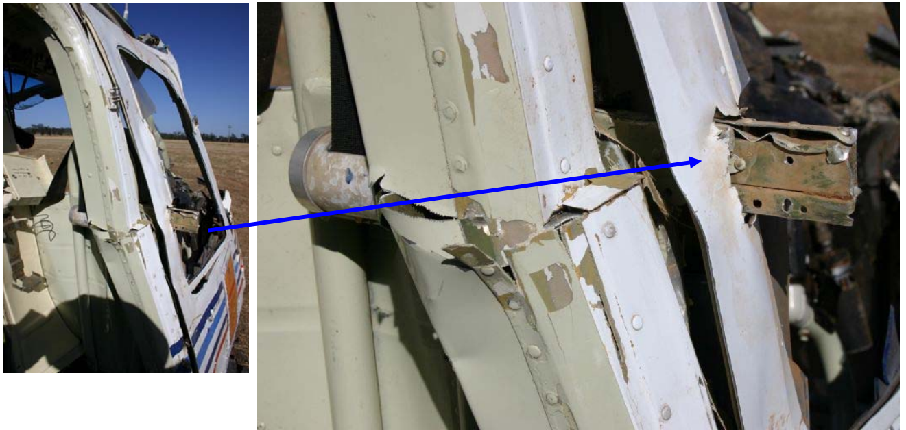
Figure 14: Horizontal beam projecting through the skin of right side cockpit door
