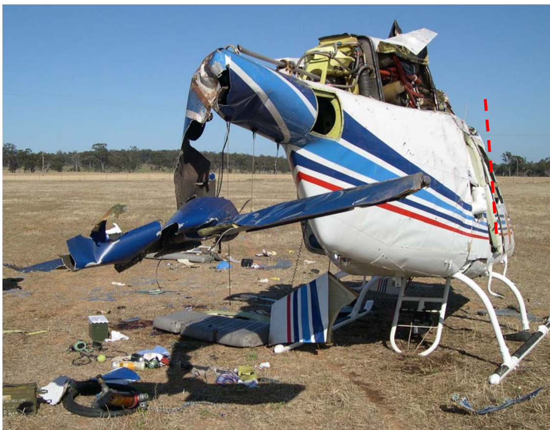
Figure 13: Distortion of fuselage structure
