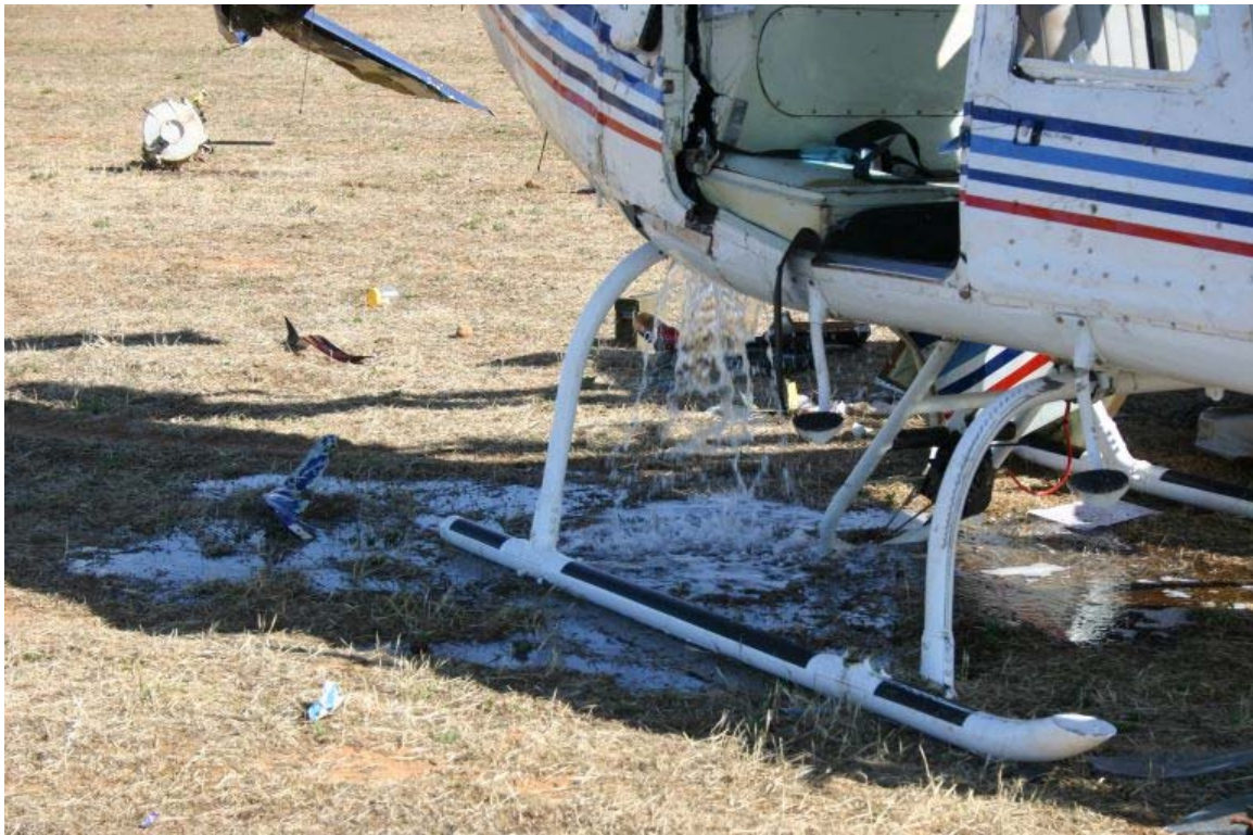
Figure 15: Disrupted fuel tank evident as helicopter is righted
