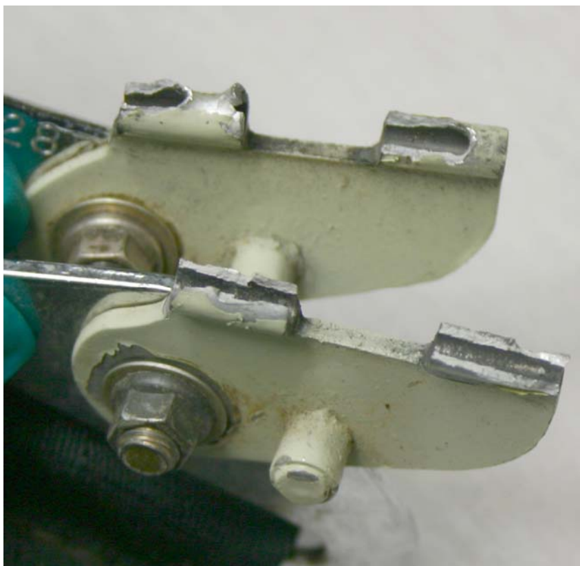
Figure 19: Failed seat belt attachments for left front crew seat
