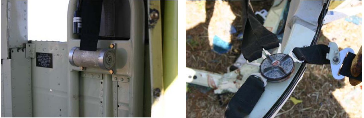
Figure 16: Front crew seat inertia reel assembly and harness buckle correctly secured
