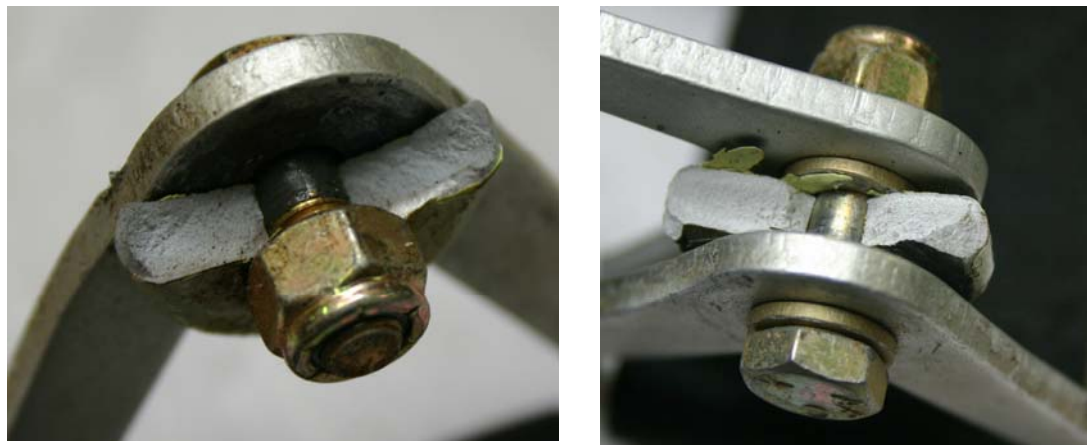
Figure 21: Failed seat belt attachments for left rear cabin seat
