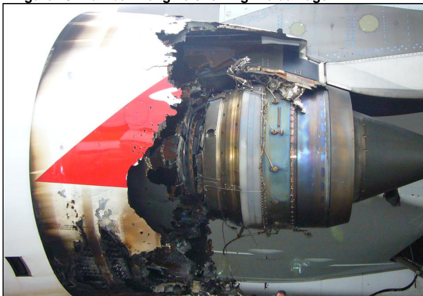
Figure 13: Number 2 engine showing fire damage
