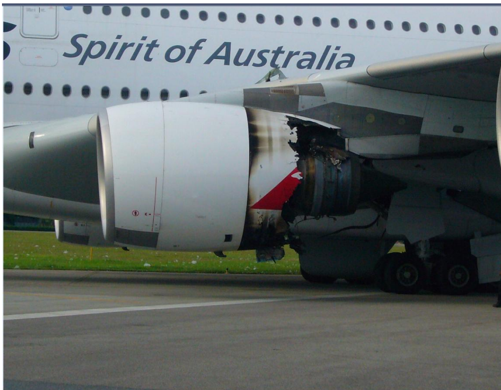
Figure 1: VH-OQA showing the damaged No 2 engine
