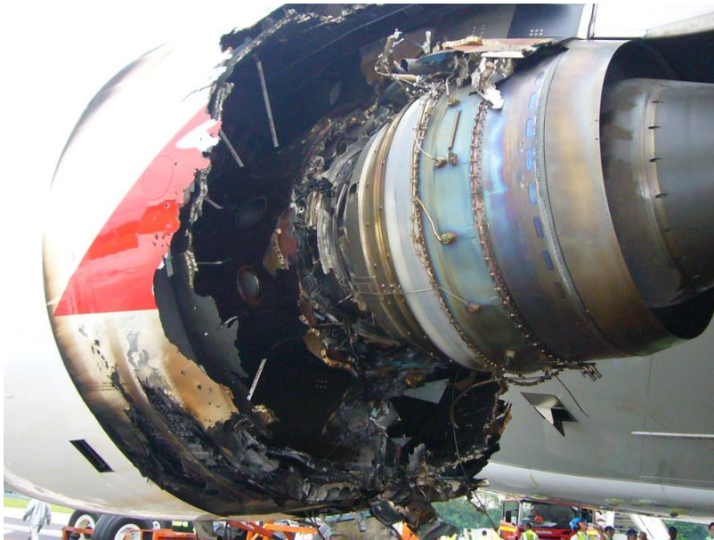
Figure 7: Damage to the No 2 engine
