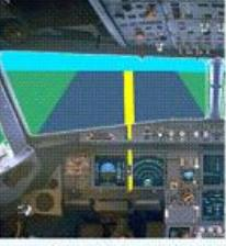
➤ On a straight taxiway, the aircraft is correctly aligned on the centerline when the centerline is lined-up between PFD and ND.
