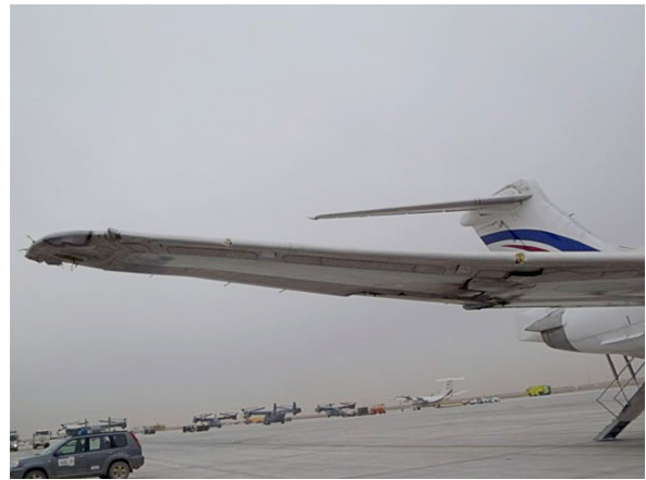
Figures 2 y 3. Damaged right wing seen from the front
