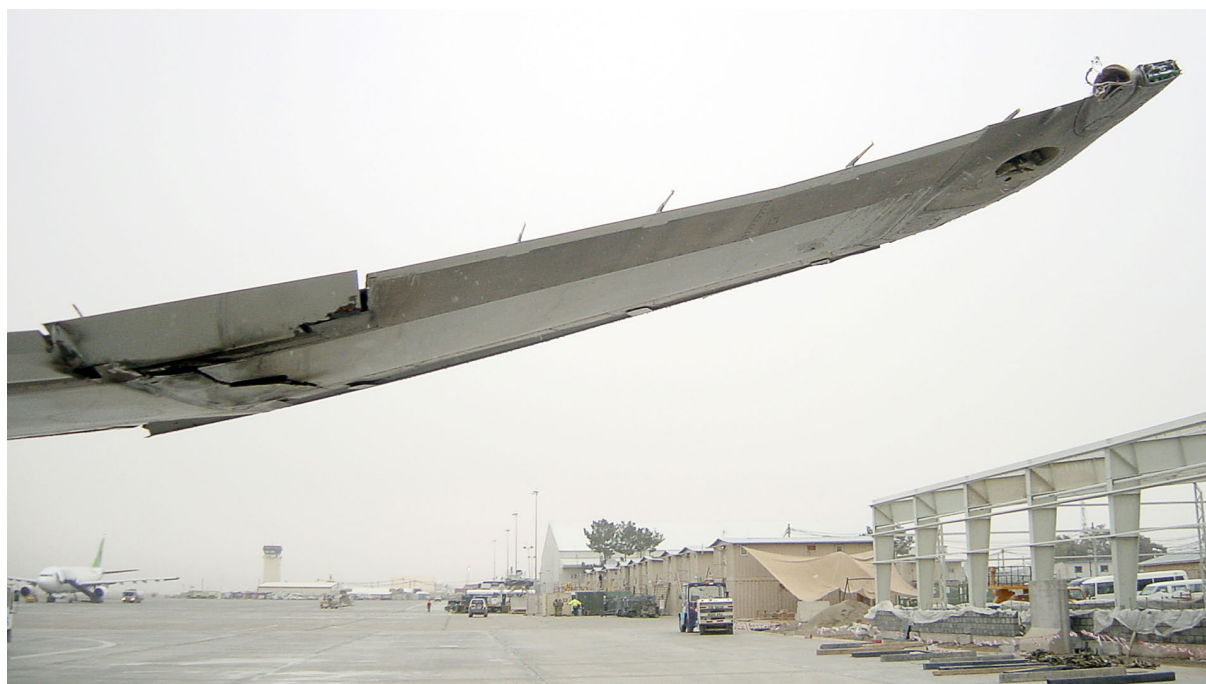
Figure 1. Damaged right wing seen from behind
