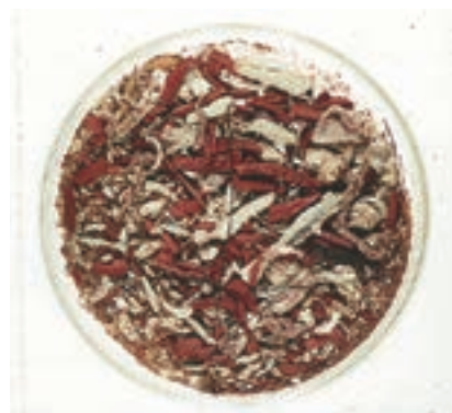
Figure 1. Sealant Material Found at the Bottom of Tank
