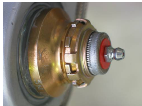
Photo of the end of the shaft with 0.5 mm of grooves visible after the washer lock.
