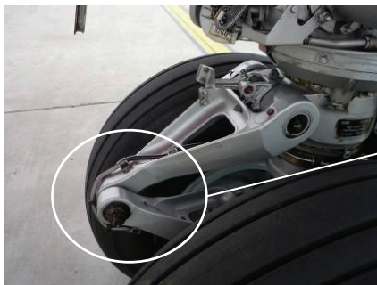
Diagram and photos (side and face views) of the NLG torque link assembly on the A300-B4
