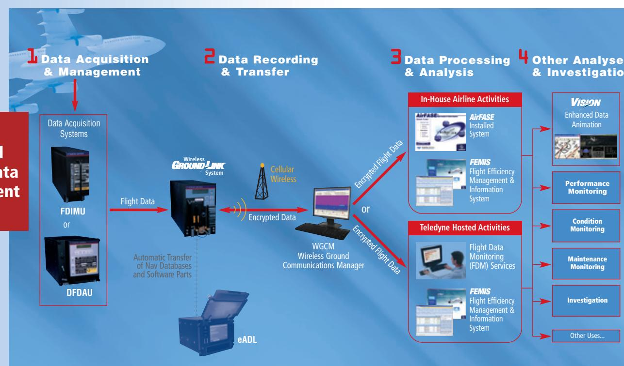
The AirFASE® software is an essential part of Teledyne Controls' end-to-end aircraft data management solutions. Designed to assist airlines with their FOQA/FDM initiatives, these offerings include innovative airborne data acquisition products, air-to-ground wireless data transfer systems and ground-based applications that fit together to deliver greater benefits to the operators and provide the total solution that airlines need for a successful flight safety program.
