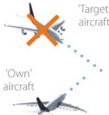
TCAS on-board the 'own' aircraft filters out the 'target' aircraft
