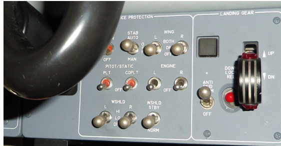
Figure 3 – ICE PROTECTION panel
