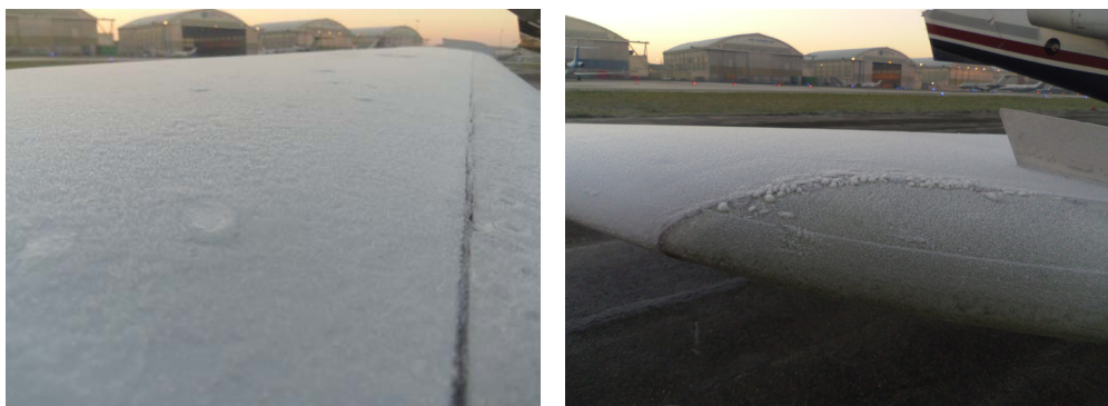
Figure 9 - Roughness on a wing contaminated by frost
