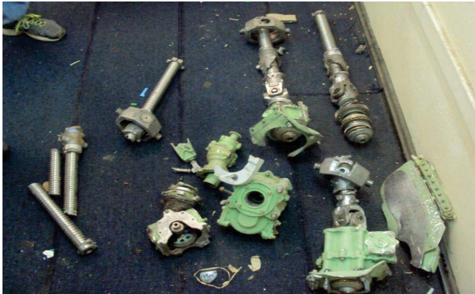
FIGURE56: TRAILING EDGE FLAP TRANSMISSIONS AND BALL SCREWS
