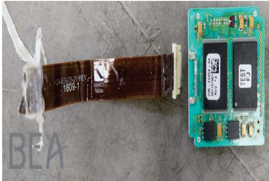
FIGURE 34: FDR MEMORY BOARD, FLEX AND CONNECTOR
