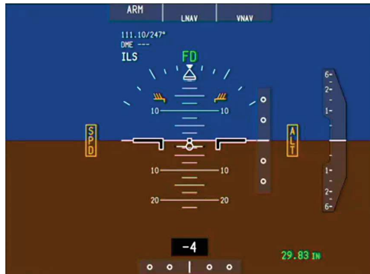
FIGURE 22: INSTRUMENT SPD AND ALT FLAGS APPEAR ON PFD
