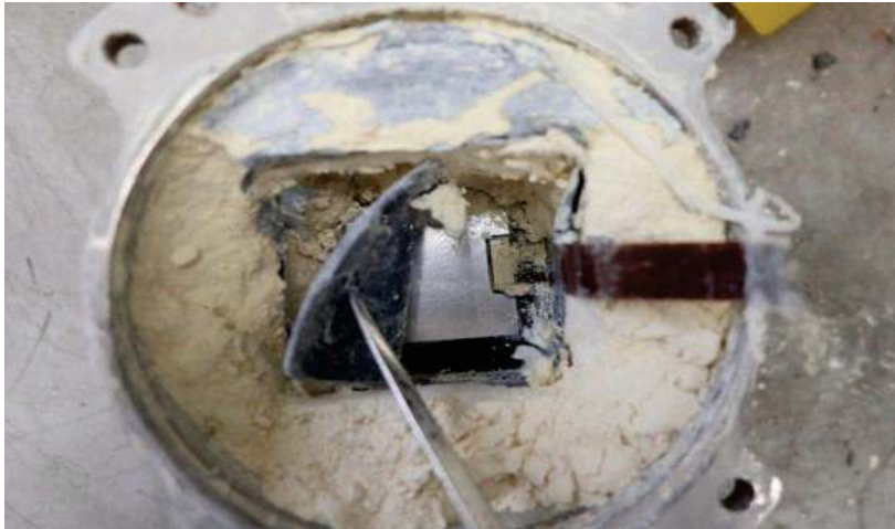
FIGURE 2: AT OPENING THE FDR CSMU, SHOWING THE MEMORY PUCK AND FLEX
