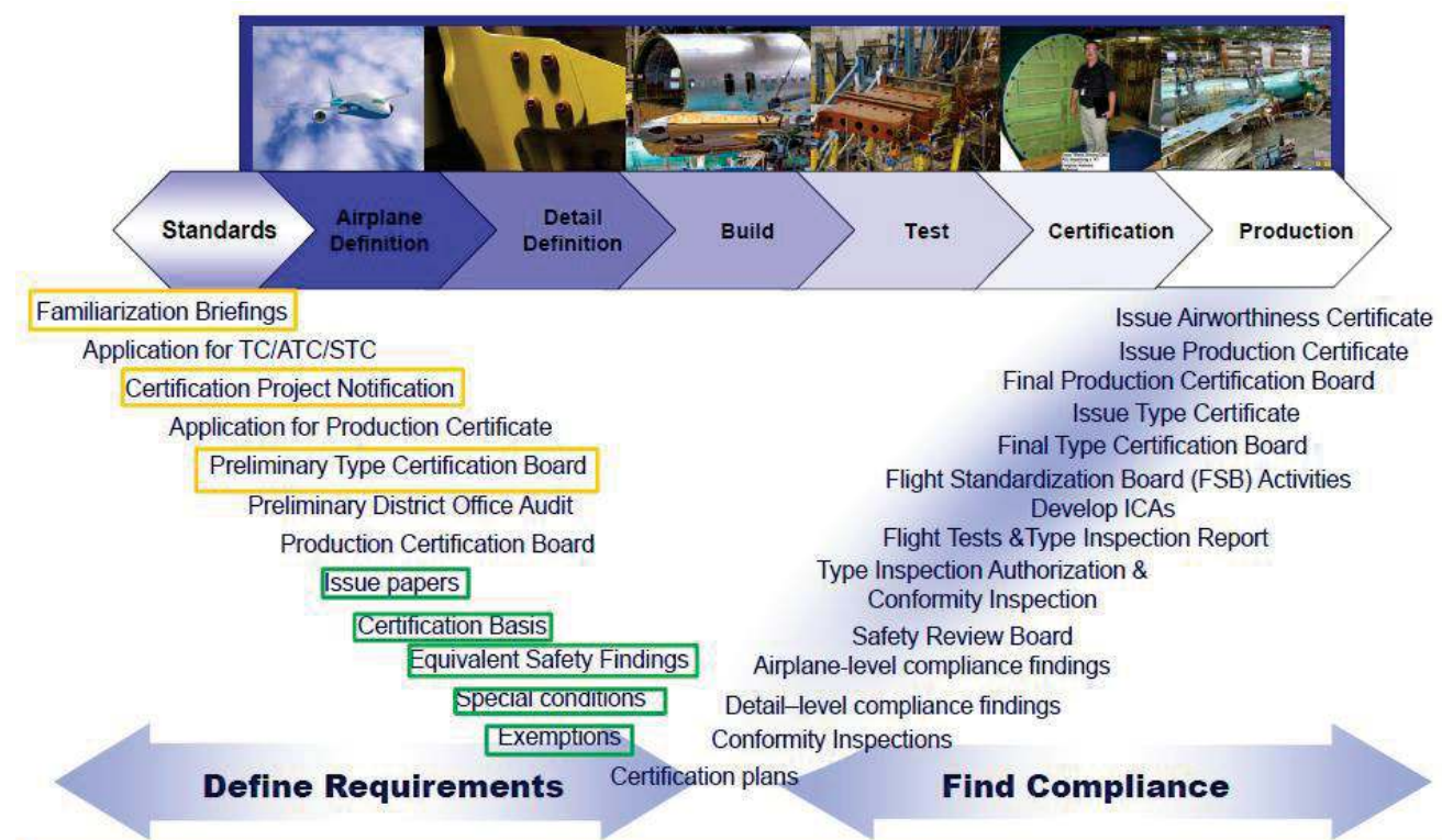
FIGURE 90: DIAGRAM OF FAA CERTIFICATION PROCESS
