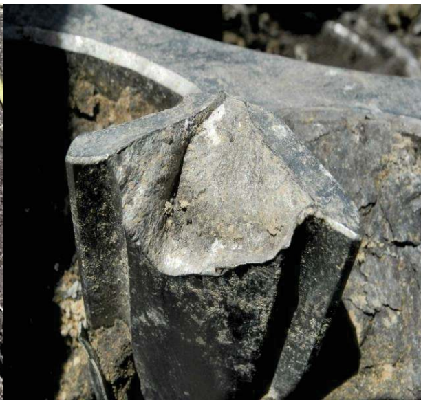
FIGURE46: R/H ENGINE - S/N 602695 - FAN DISK FIGURE47: R/H ENGINE - S/N 602695 - RETENTION LUGS - FRACTURED
