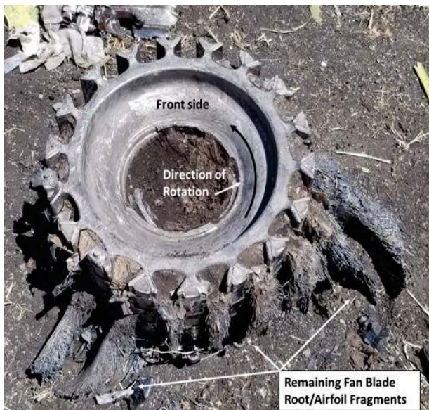
FIGURE46: R/H ENGINE - S/N 602695 - FAN DISK FIGURE47: R/H ENGINE - S/N 602695 - RETENTION LUGS - FRACTURED
