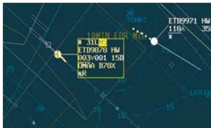
Figure 8. Radar screenshot - Aircraft at two nautical miles on final approach, indicated altitude 300 feet (corrected), and activation of minimum safe altitude warning [Source: GAL ANS]
