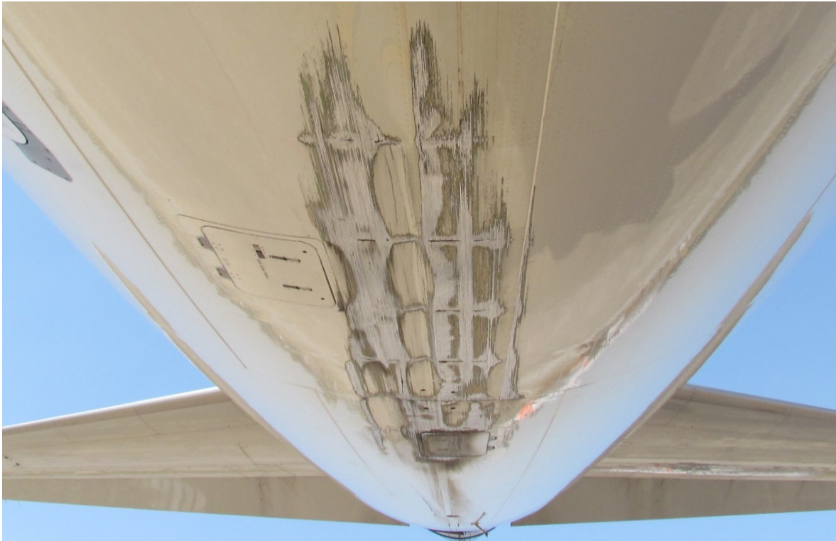
Figure (4) Scrape marks on aircraft tail section
