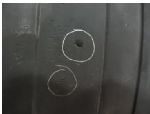
Figure 16. Cuts on wheel number 6 (paired with no. 5), produced on 30/01/2020
