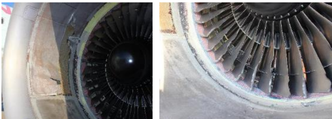
Figure 15. Damage to the fan
