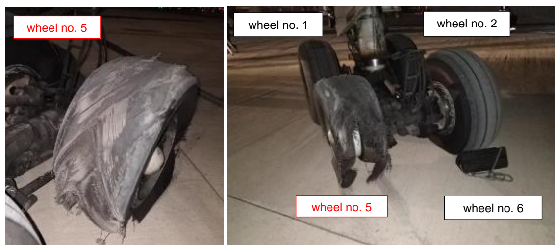
Figure 5. Left main landing gear (seen from behind) after the landing
