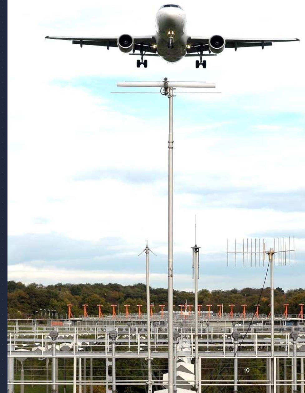
Orbital and radial measurement flights for preventive and corrective maintenance as well as preparation for commissioning.
