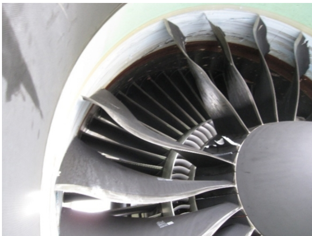
Photo 1: Fractured Fan Blade at Platform
