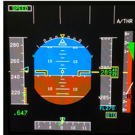
Figure 20: PFD with vertical speed tape indicating a Climb RA on an Airbus A320.
