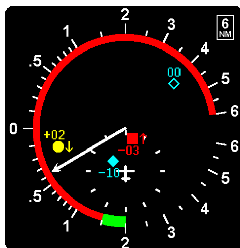
Figure 13: Traffic display example – IVSI combined with traffic display.
