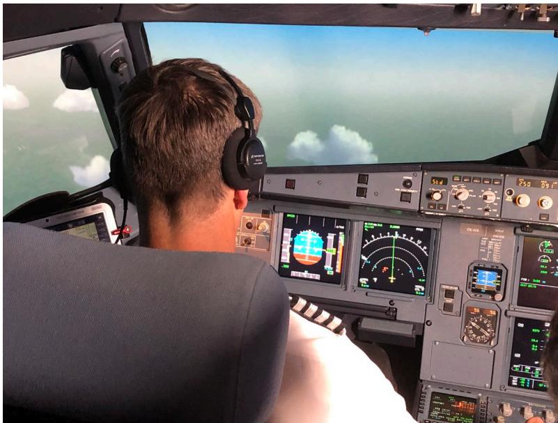
Figure 21: Primary Flight Display (left) and Navigation Display positions on Airbus A320.
