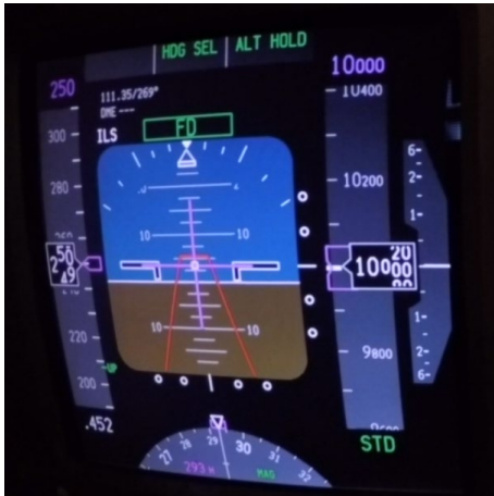
Figure 19: PFD with pitch cue display indicating a Climb RA on a Boeing 737-800.
