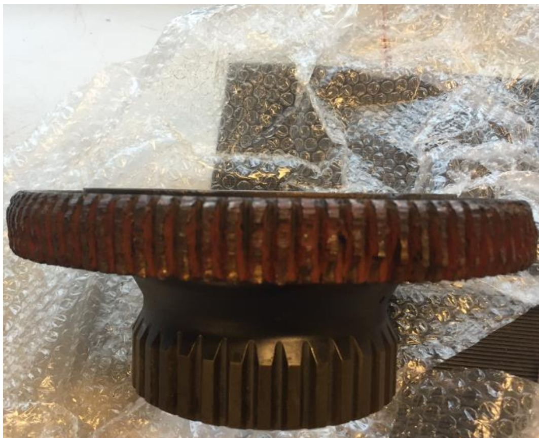
Figure 8: First stage Sun Gear. Photo: AIBN
