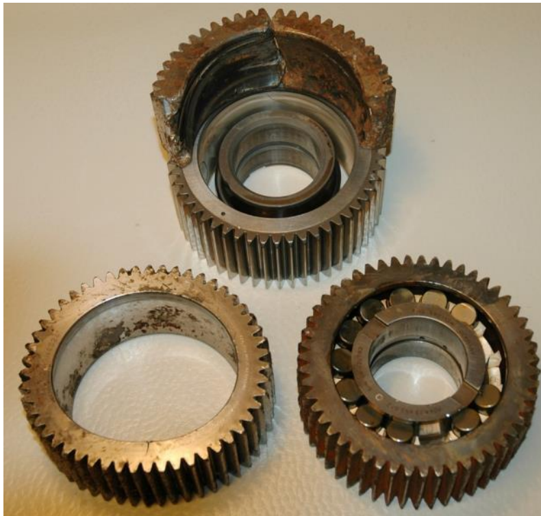
Figure 2: Planet gear parts from second stage epicyclic reduction gear module. (The fractured gear is on top of a sample gear that was not involved in the accident.) Photo: AIBN
