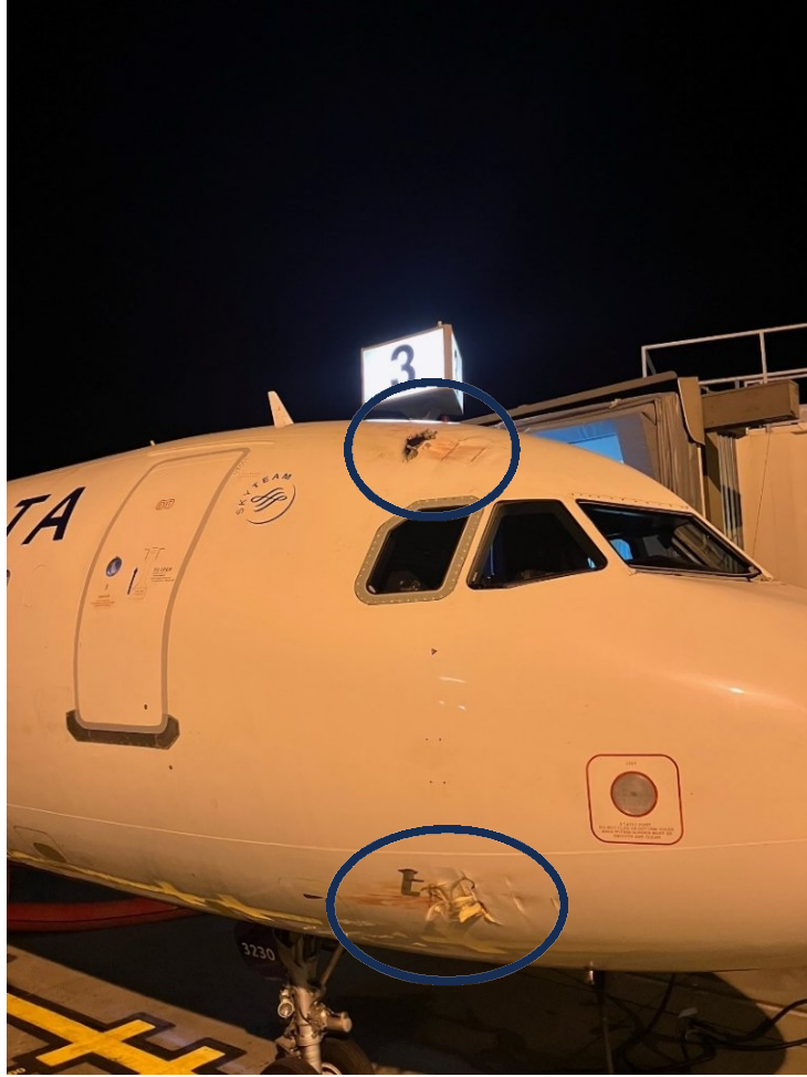
Figure 1. Photo of two of the bird strikes on the left side of the airplane, indicated by blue circles. (Source: Delta Air Lines)
