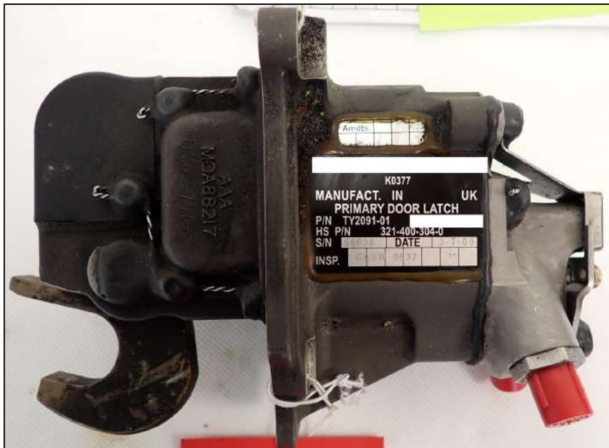
Figure 17. A PDL in as received condition
