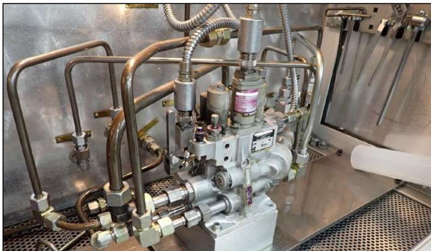
Figure 18. HCU in test rig
