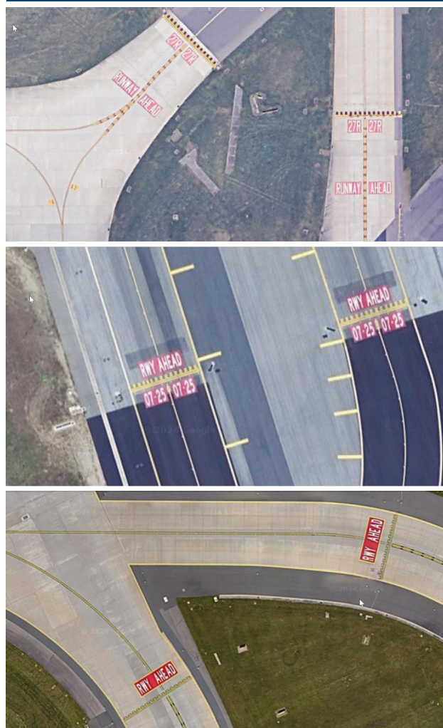
Figure 6. Example of 'RWY AHEAD' markings
