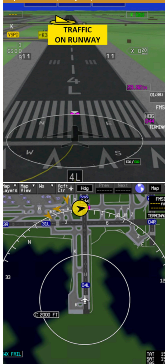
Figure 42. Example of SURF-IA prototype implementation (Honeywell).
