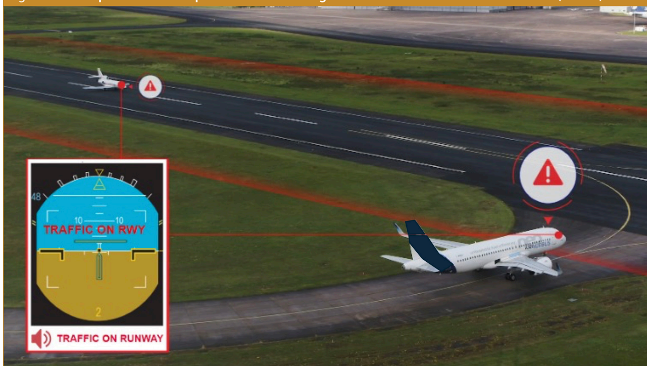
Figure 43. Example of SURF-A implementation showing a PFD - and the associated audio - alert (Airbus).
