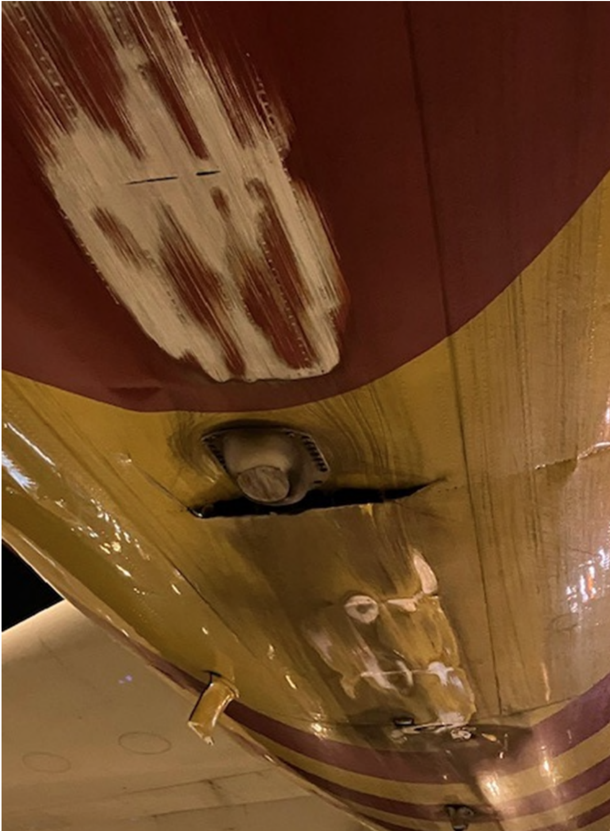
Fig. 9: Damage at the outer skin / covering at the lower aft fuselage
