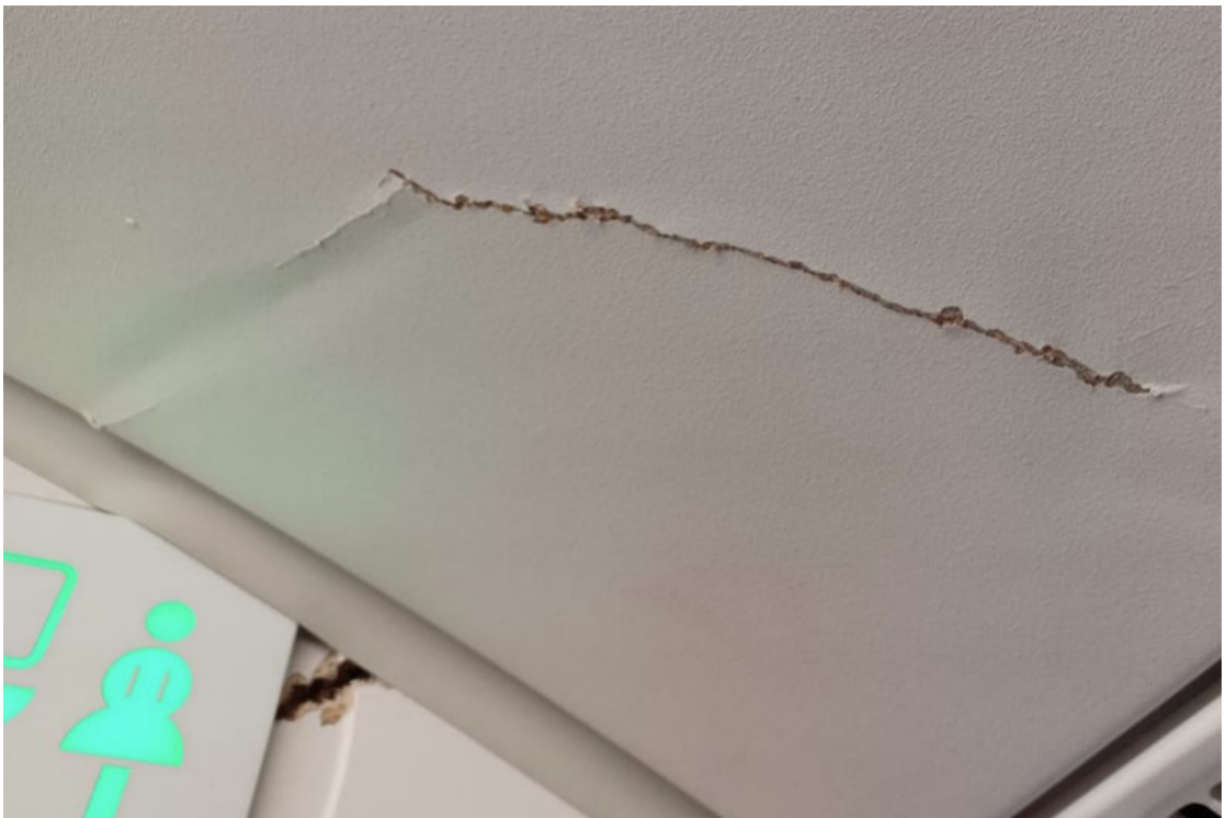
Fig. 19: Damage in the area of the ceiling lining, row 46
