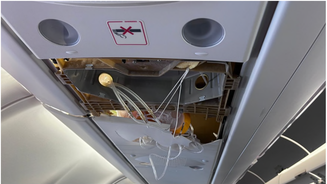
Fig. 18: Damage on passenger service units
