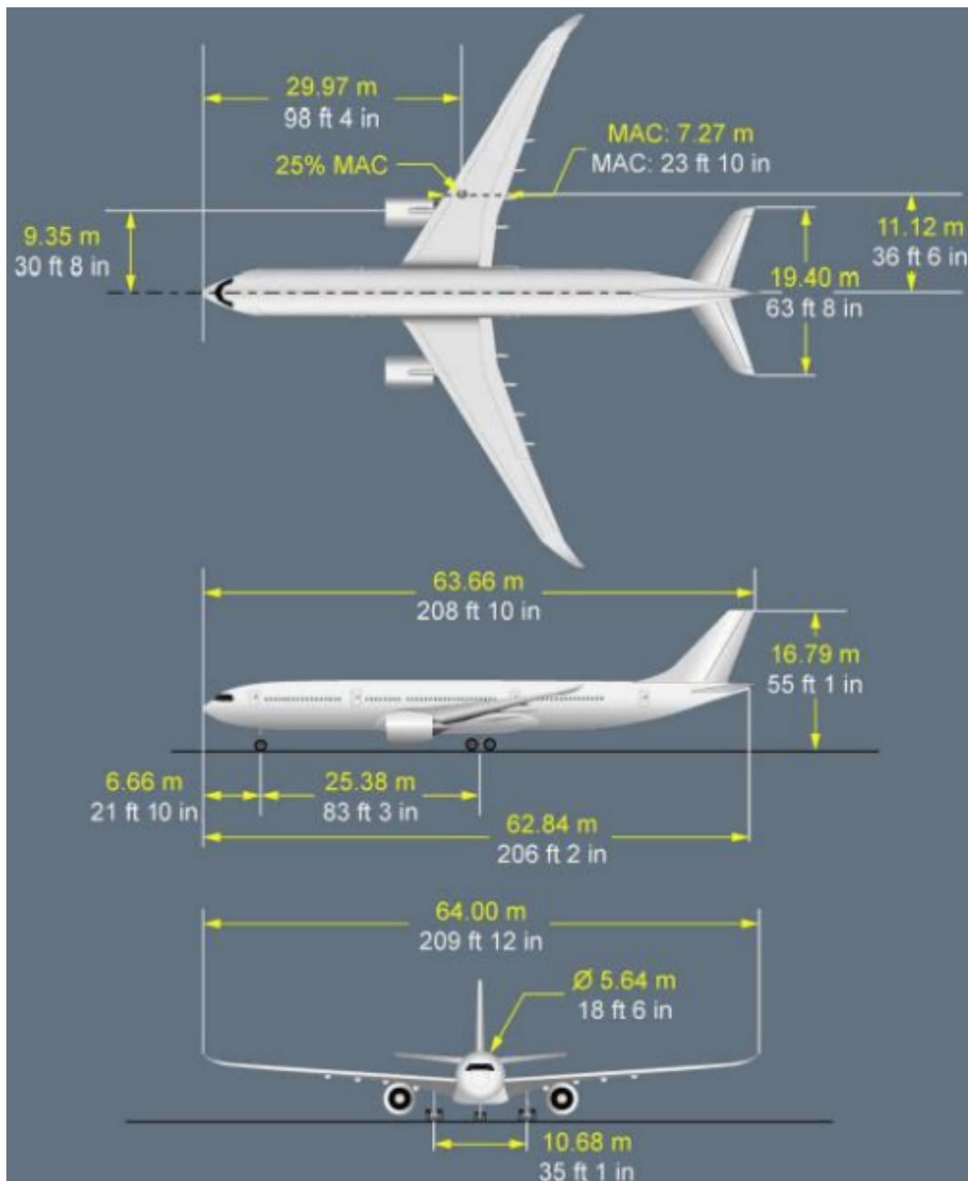
Fig. 1: Three-way view of the Airbus A330-941
