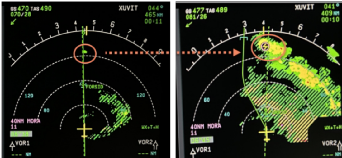
Weather display at 120 Nm from Weather condition [left] and at 70 Nm from Weather condition [right]
