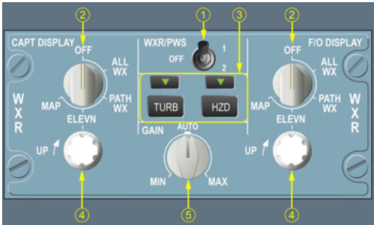
Fig. 6: Control panel and switch designation of the weather radar RDR-4000.
