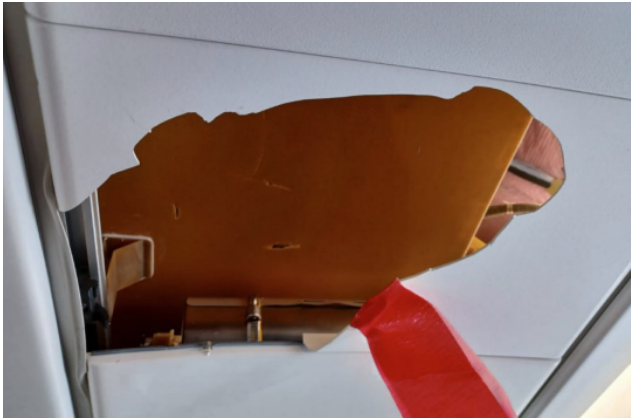
Fig. 20: Damage in the area of the ceiling lining, row 23 HK
