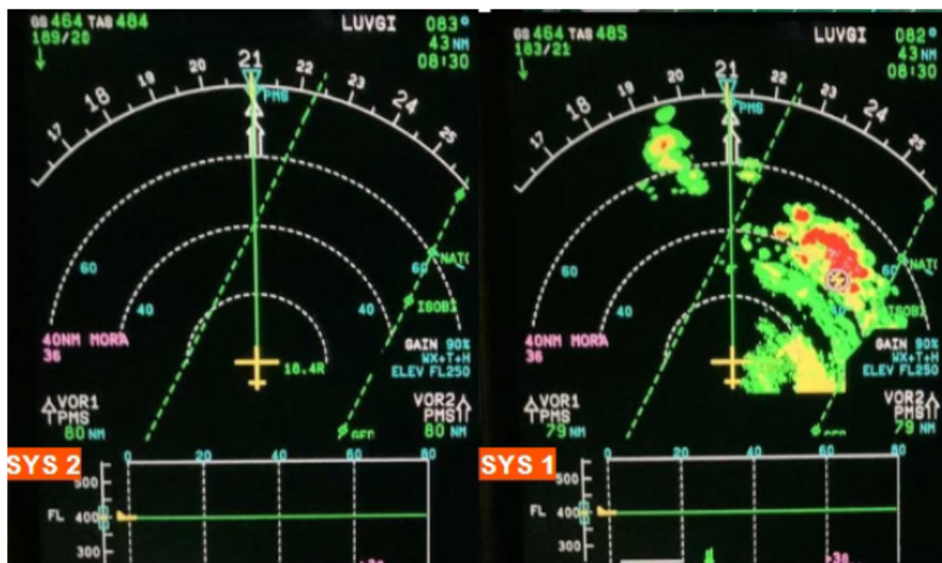
Comparison between degraded and healthy WXR system at same area, time and settings
